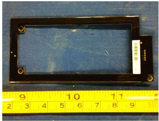
High Frequency Long Antenna Bottom View
