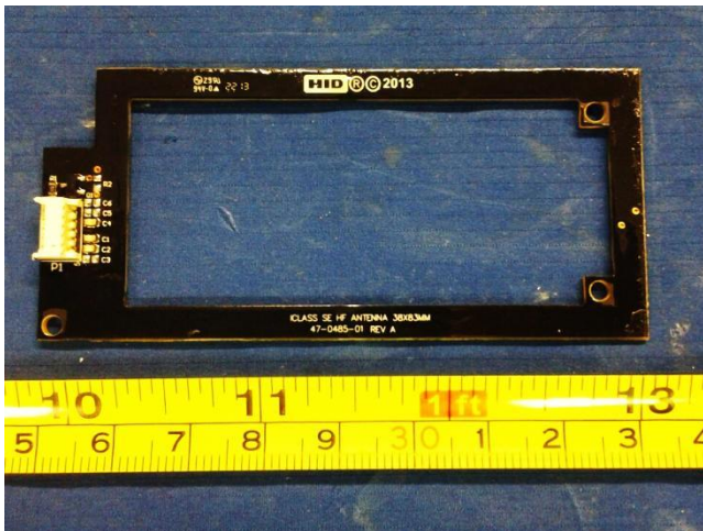
High Frequency Long Antenna Top View
