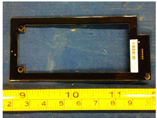
High Frequency Long Antenna Bottom View
