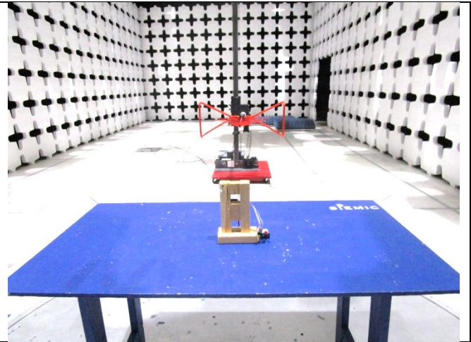
Radiated Emissions (<1GHz) – Rear View
