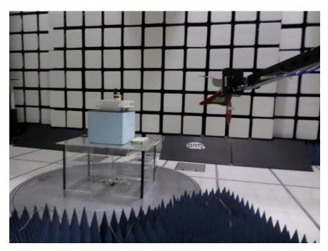
Photograph 4. Radiated Emissions, Setup Above 1GHz, Antenna view
