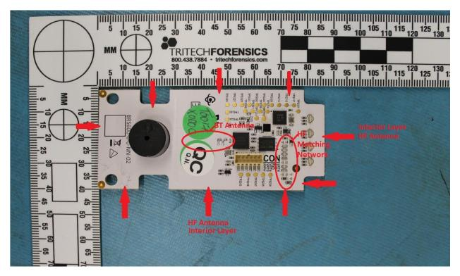
Note: Both the HF (13.56 MHz and BLE Antenna's are on internal layers)
