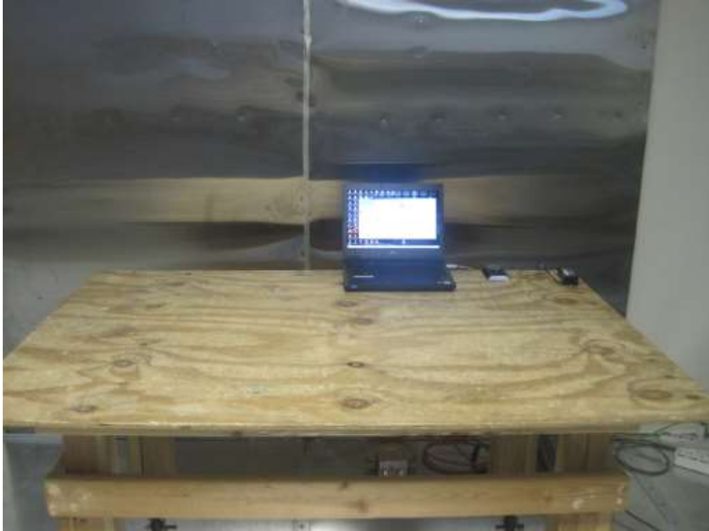
AC Line Conducted Emission Set up
