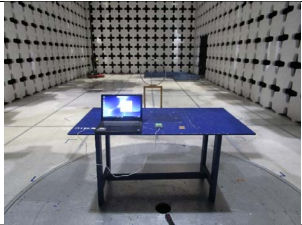
Radiated Emissions (<30MHz) – Rear View
