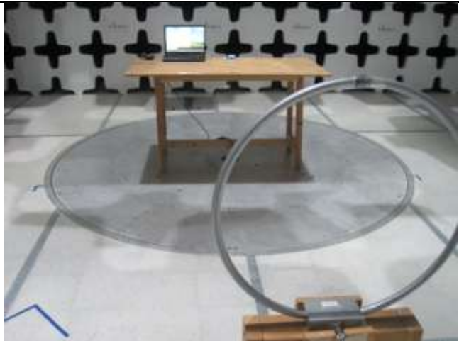
Radiated Emission Test setup (<30MHz) - Front
