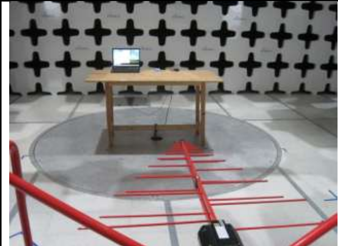
Radiated Emission Test setup (<1GHz) - Front
