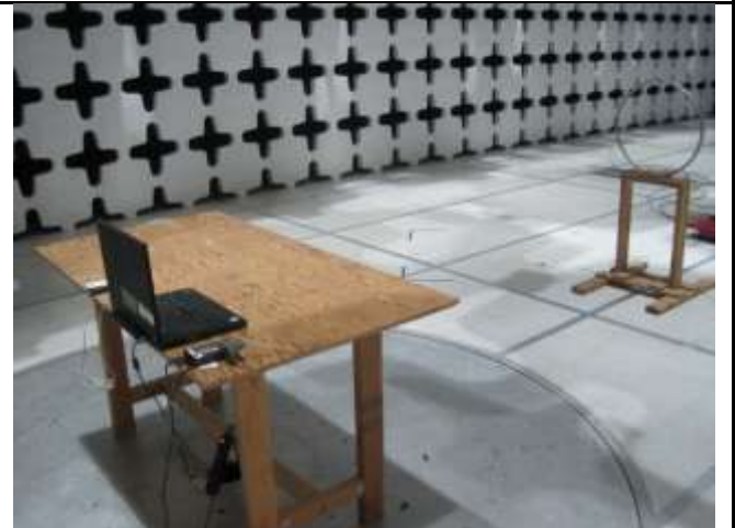
Radiated Emission Test setup (<30MHz) - Rear
