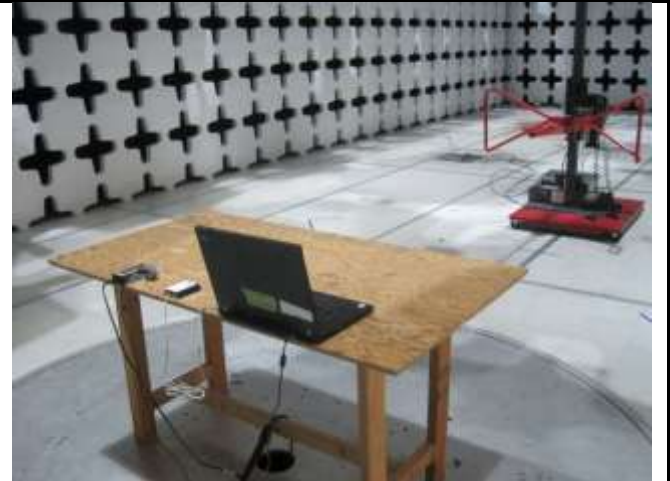
Radiated Emission Test setup (<1GHz) - Rear
