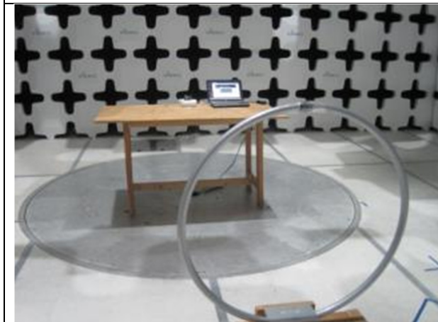
Radiated Emissions Test setup (<30MHz) – Front View
