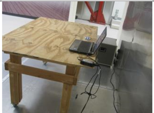
Conducted Emission Test setup - Rear
