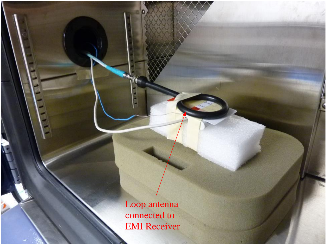
Figure 10: Frequency Stability Test Setup (Close-up)
