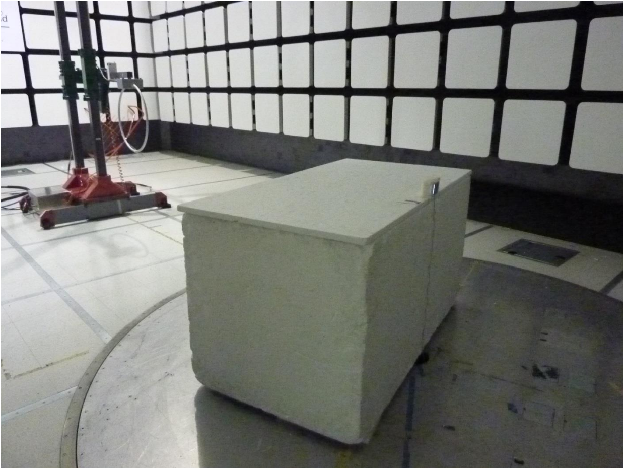
Figure 5: Test Setup for 9 kHz to 30 MHz; antenna at 90 degrees (Mode 1)
