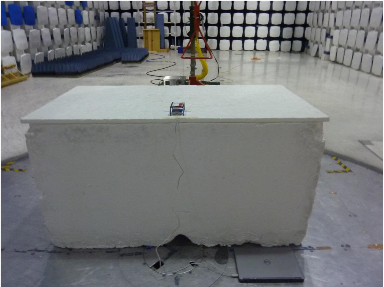
Figure 8: Test Setup for 30 MHz – 1000 MHz (Mode 2)
