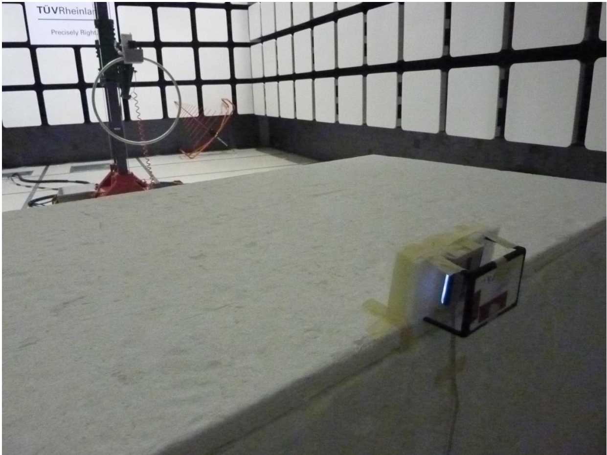
Figure 4: Test Setup for 9 kHz to 30 MHz; antenna at 0 degree (Mode 2)
