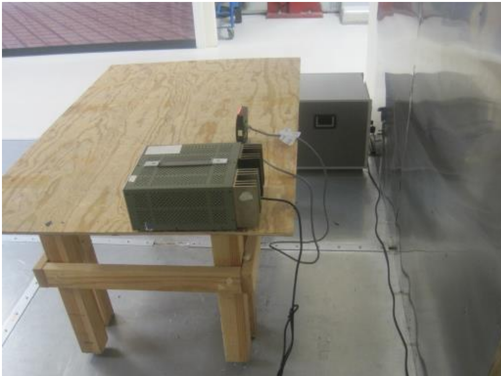
Conducted Emissions Rear View – Terminal Connector
