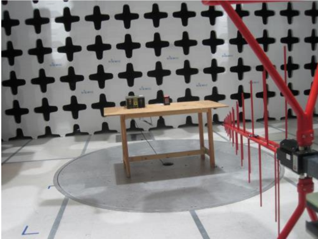
Radiated Emissions (<1GHz) Front View – Terminal Connector
