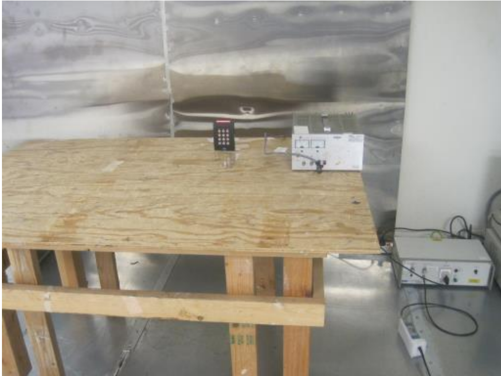
Conducted Emissions Front View – Terminal Connector
