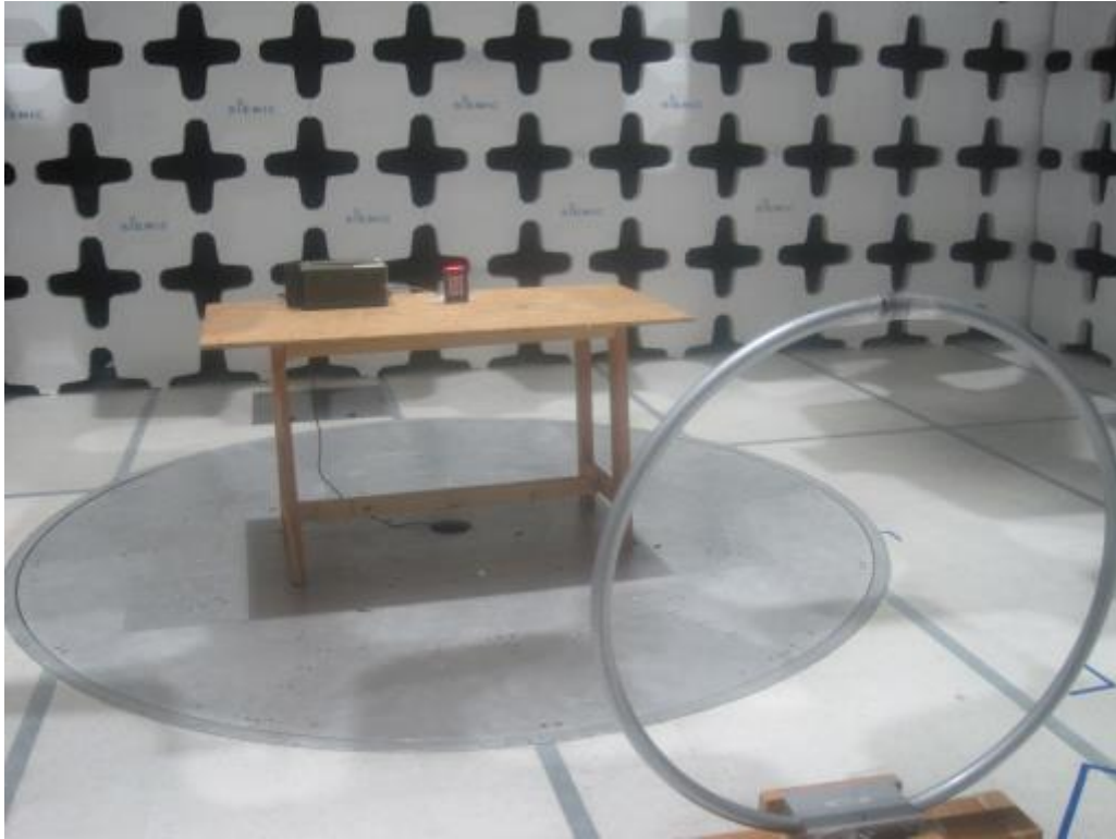
Radiated Emissions (<30MHz) Front View – Pigtail Connector
