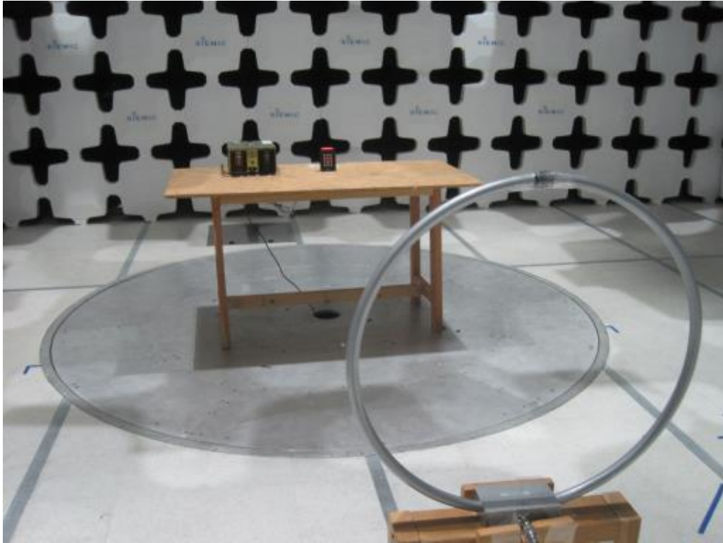
Radiated Emissions (<30MHz) Front View – Terminal Connector
