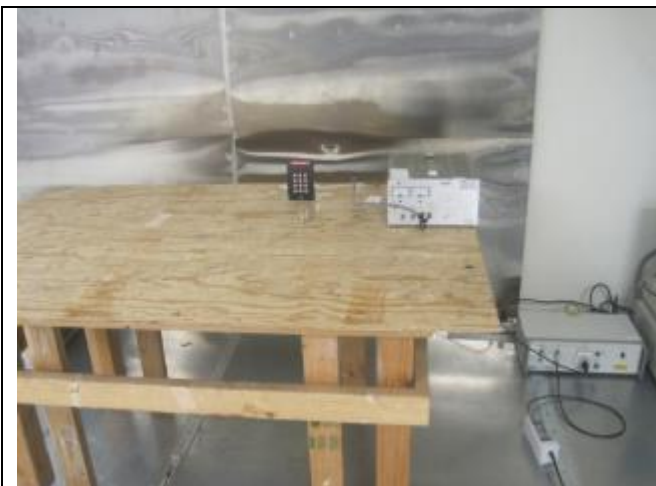
Conducted Emissions– Front View (Terminal Connector)
