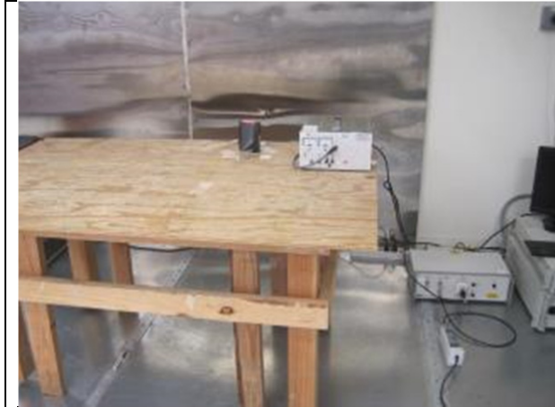
Conducted Emissions Test setup – Front View
