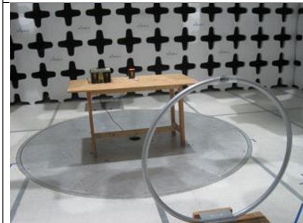
Radiated Emissions Test setup (<30MHz) – Front View
