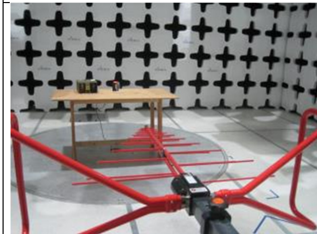
Radiated Emissions Test setup (<1GHz) – Front View
