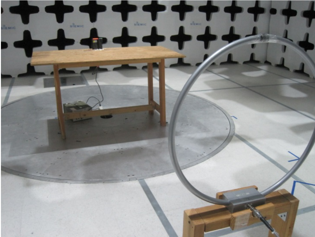
Terminal Radiated Emission<30MHz Test Setup – Front View
