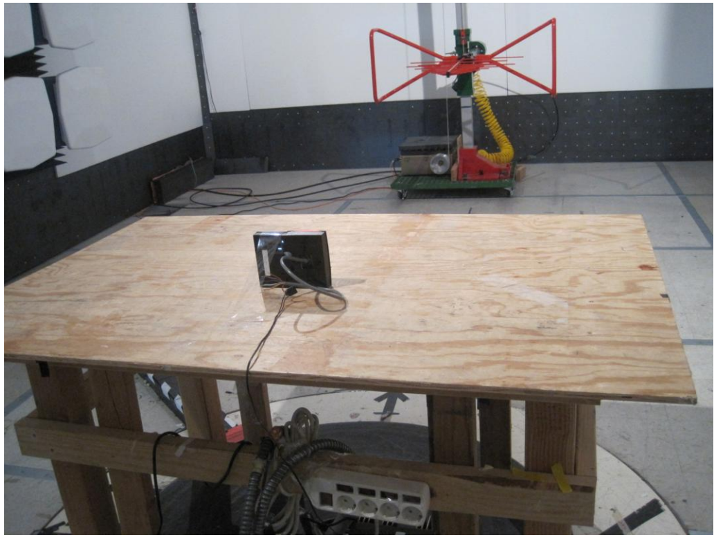
Radiated Emission Test Setup – Rear View ( Pig-Tail Connectors)
