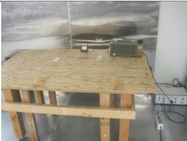
Conducted Emissions– Front View (Pigtail Connector)
