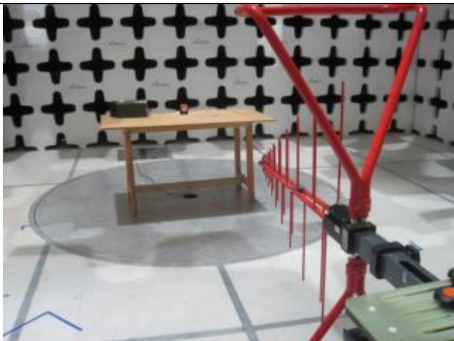
Radiated Emissions (<1GHz) – Front View (Pigtail Connector)
