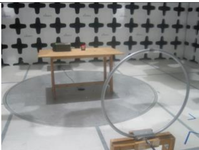
Radiated Emissions (<30MHz) – Front View (Pigtail Connector)
