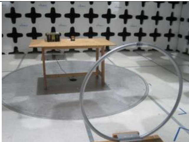
Radiated Emissions (<30MHz) – Front View (Terminal Connector)
