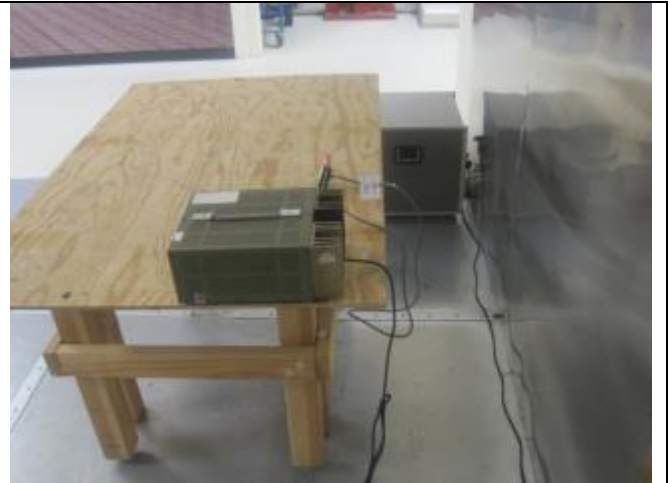
Conducted Emissions– Rear View (Terminal Connector)
