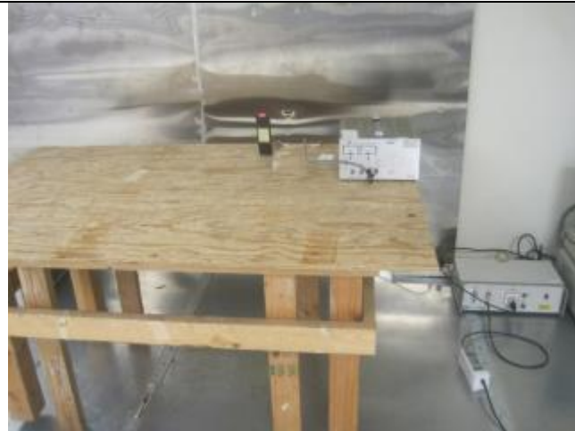
Conducted Emissions– Front View (Terminal Connector)
