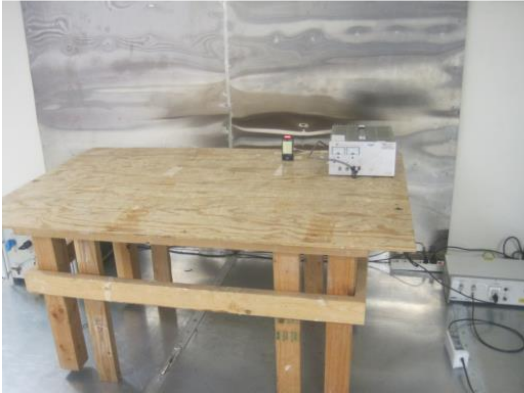
Conducted Emissions Front View – Terminal Connector
