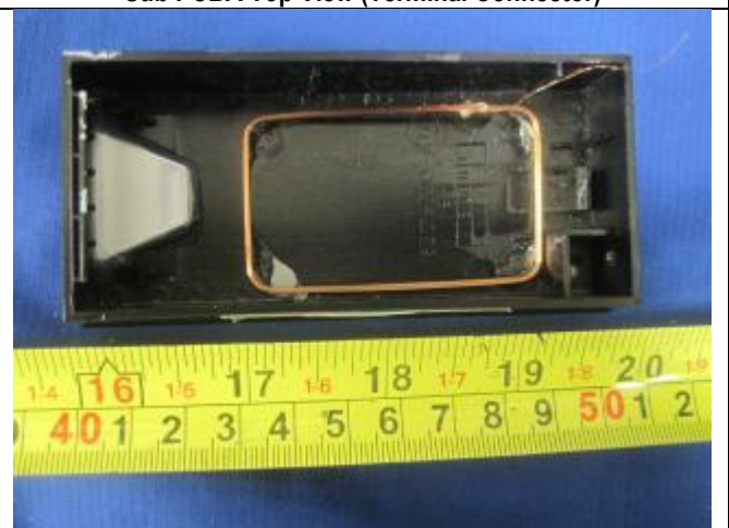
Loop Antenna (Terminal Connector)
