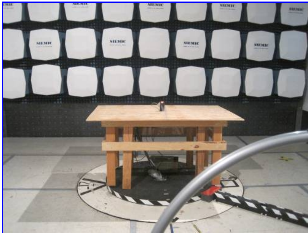
Radiated Emission (<30MHz) – Front View
