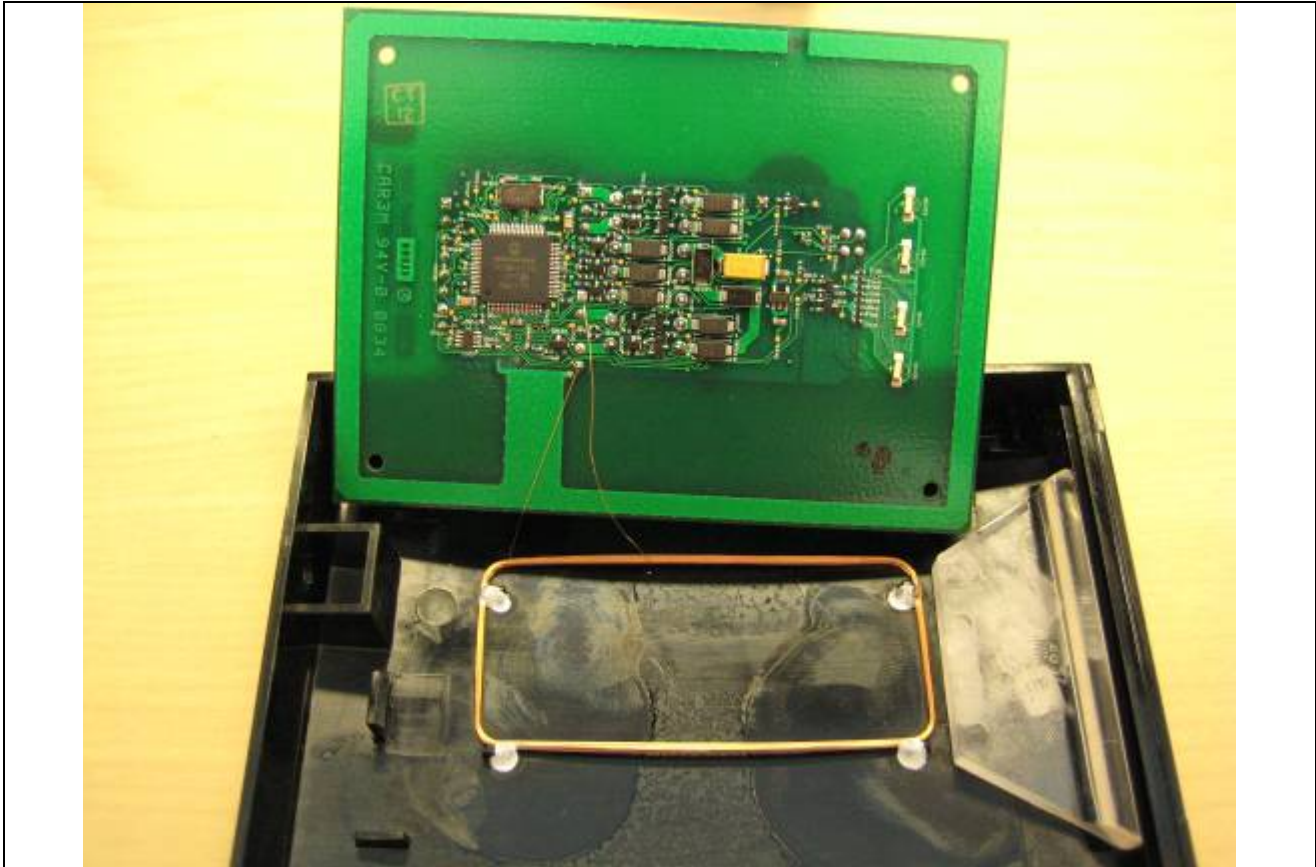
Reader Board in Plastic Housing with Antenna – Not Potted
