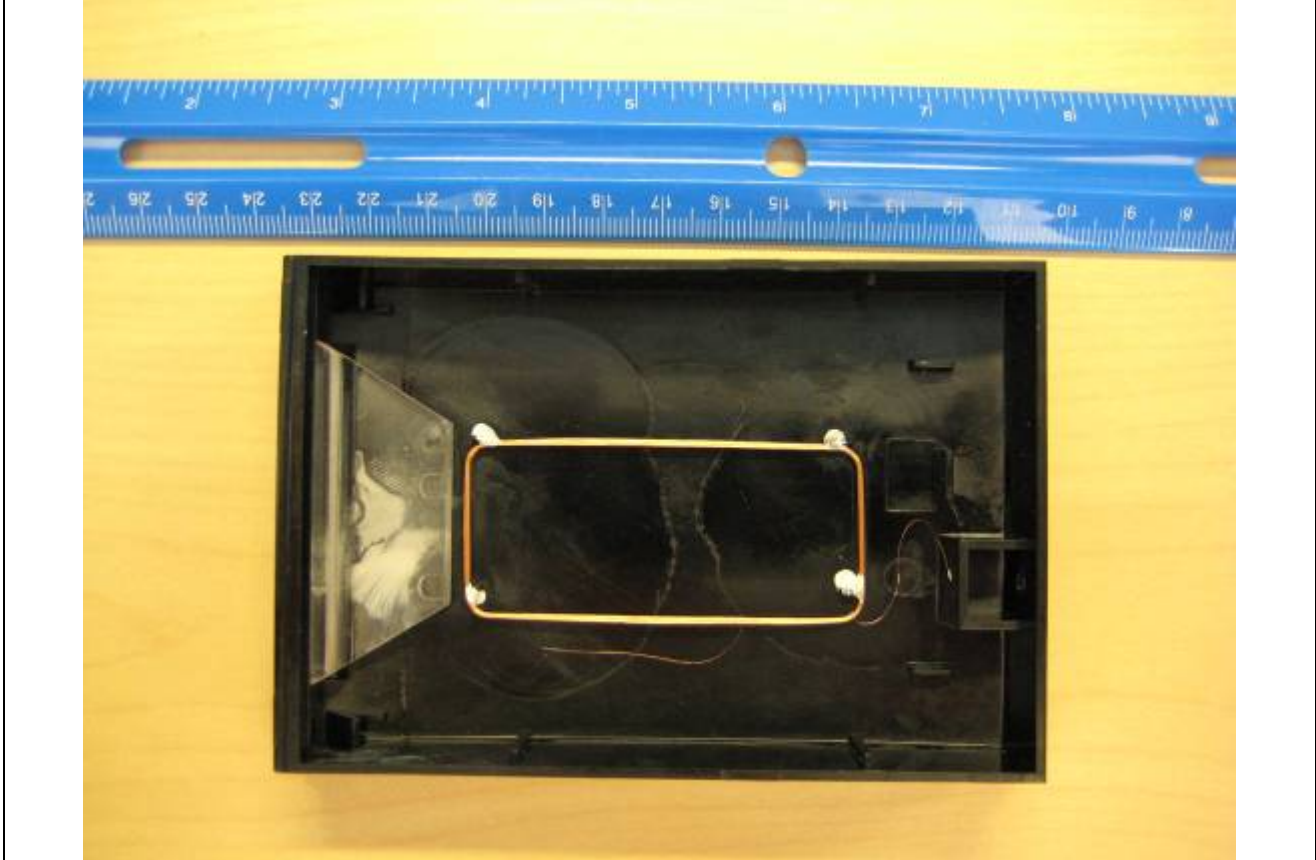
Antenna in Plastic Housing after Reader Board Removed
