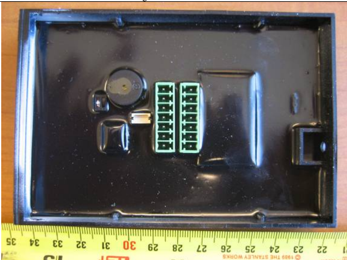
Reader Board in Plastic Housing – Potted
