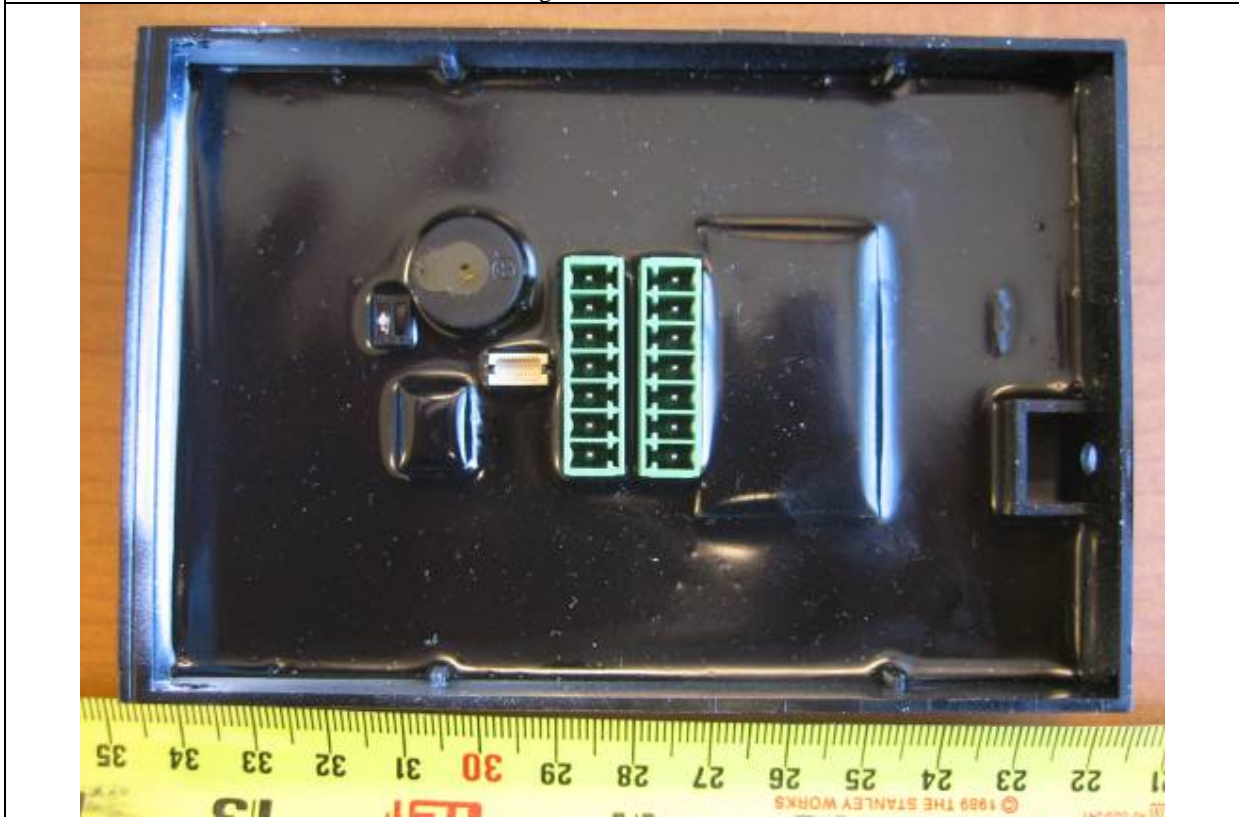
Reader Board in Plastic Housing – Potted
