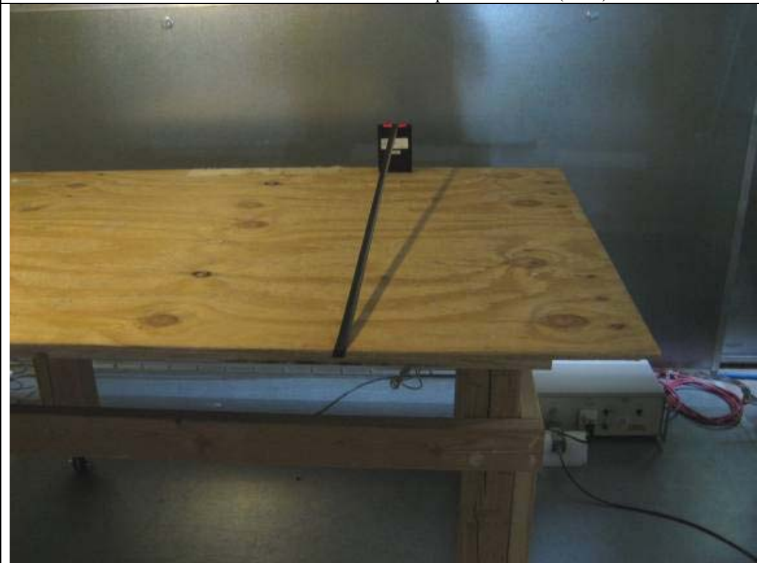
AC Line Conducted Emission Test Setup – Front View 2 (RP40)
