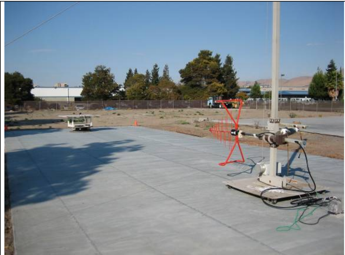
Radiated Emission Test Setup – Front View (>30MHz)
