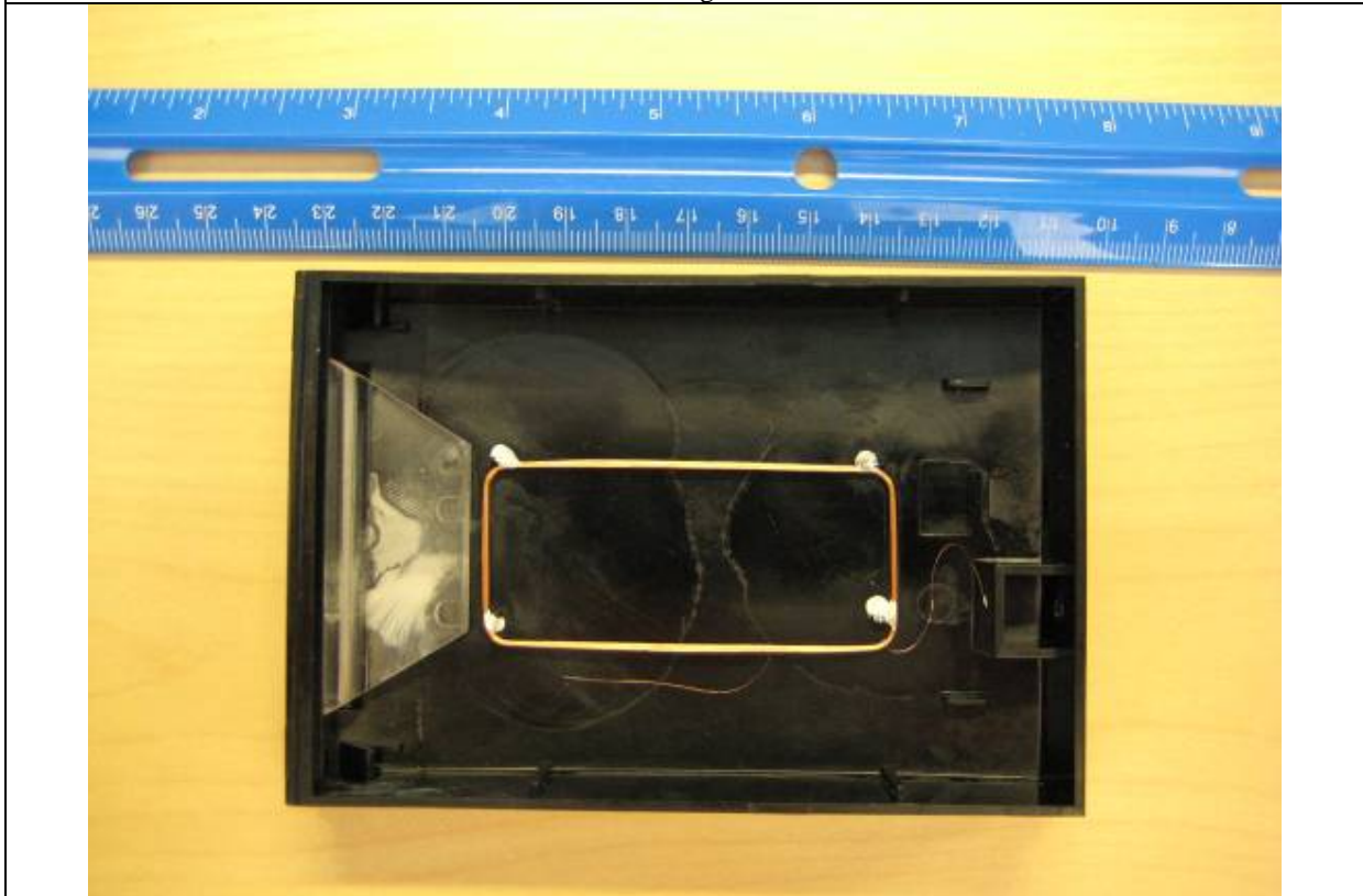
Antenna in Plastic Housing after Reader Board Removed
