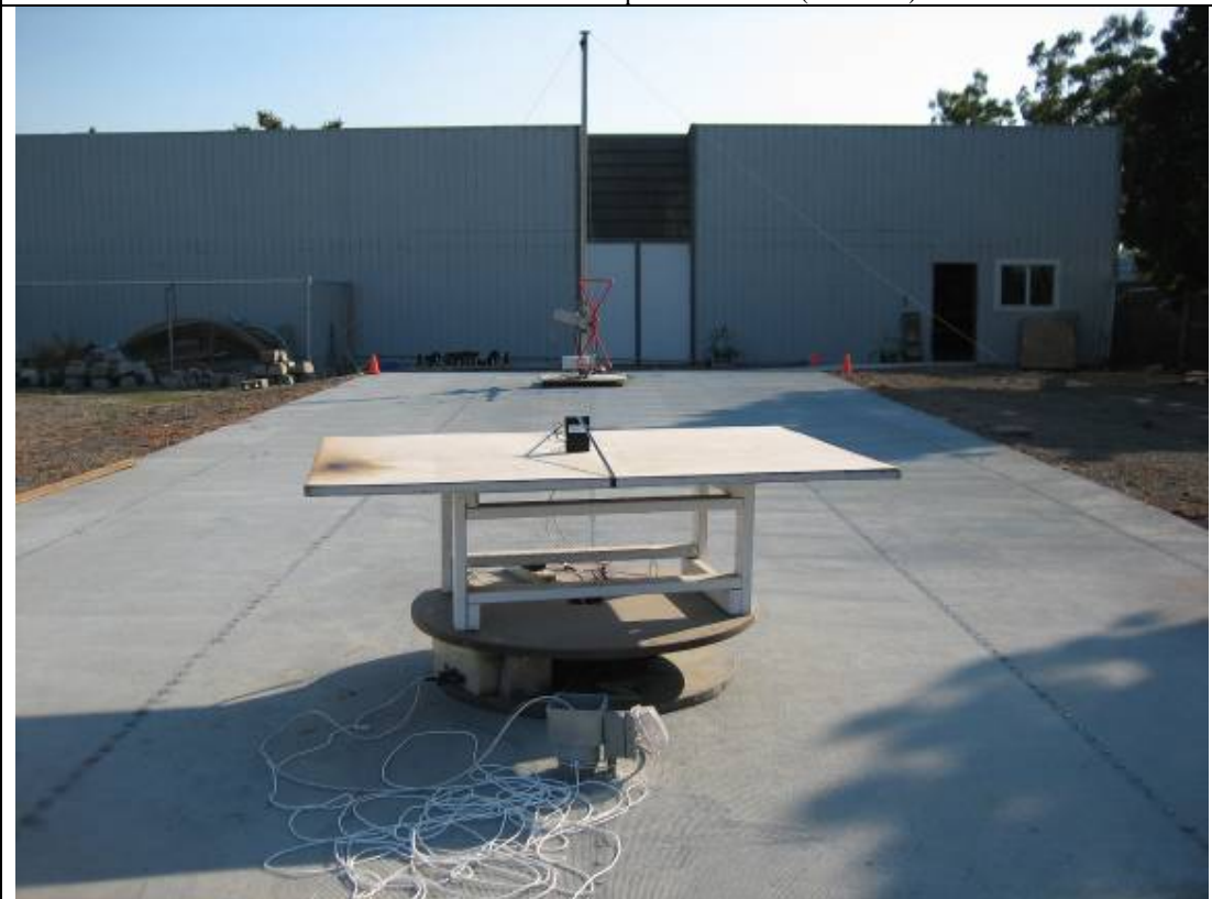
Radiated Emission Test Setup – Rear View (>30MHz)
