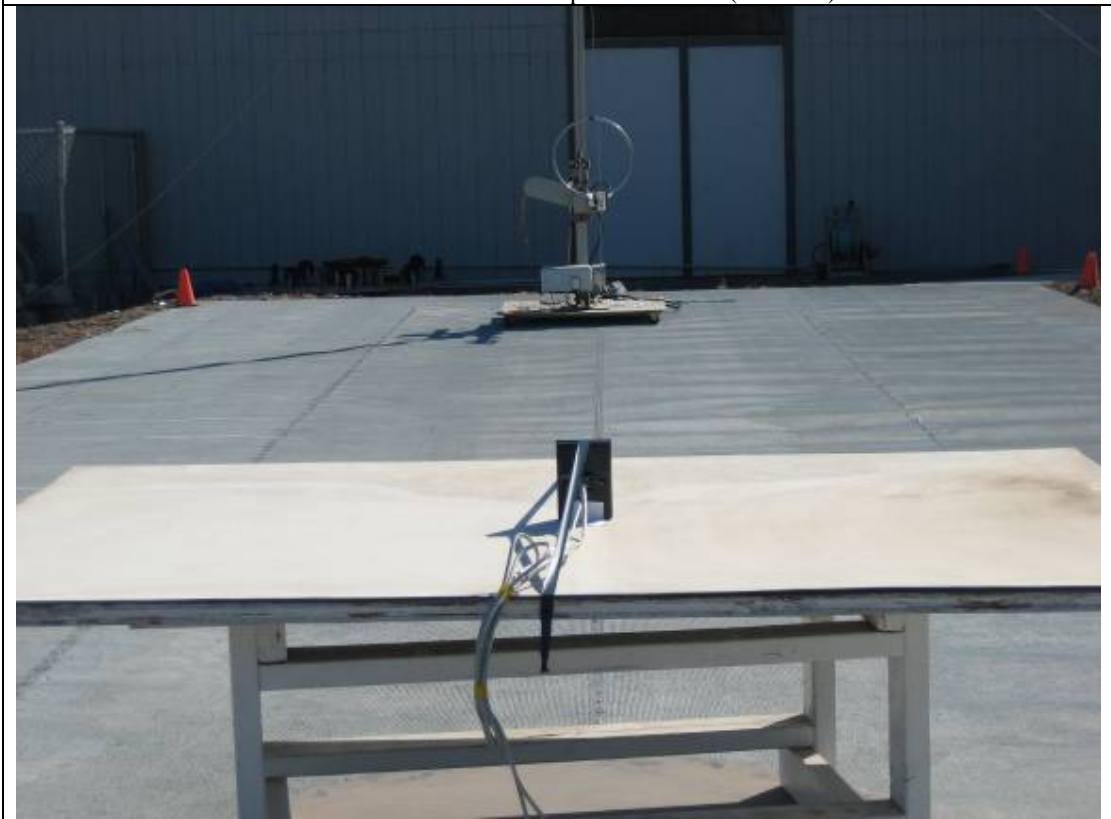
Radiated Emission Test Setup – Rear View (<30MHz)
