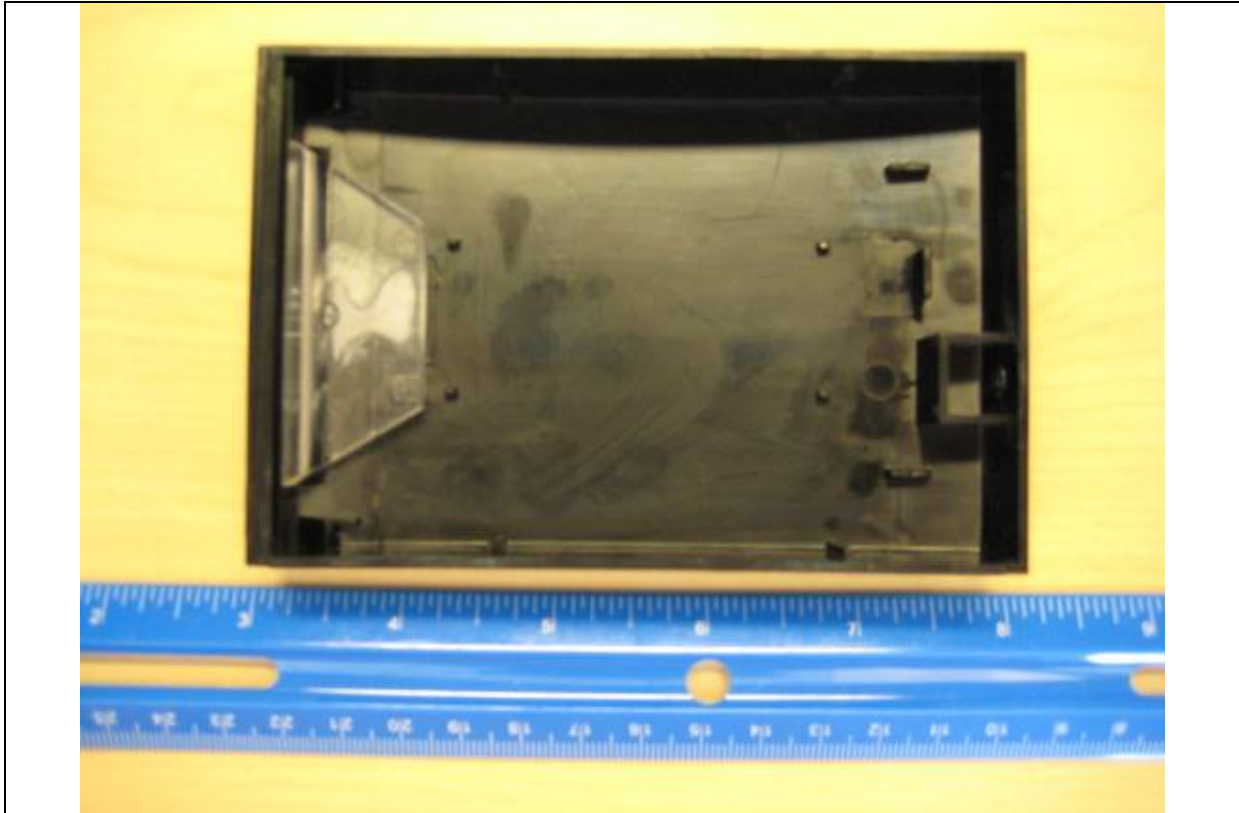
Plastic Housing after Reader Board Removed
