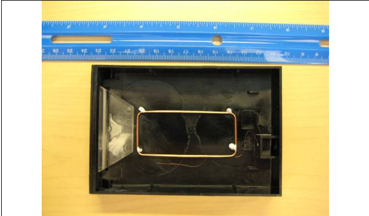
Antenna in Plastic Housing after Reader Board Removed
