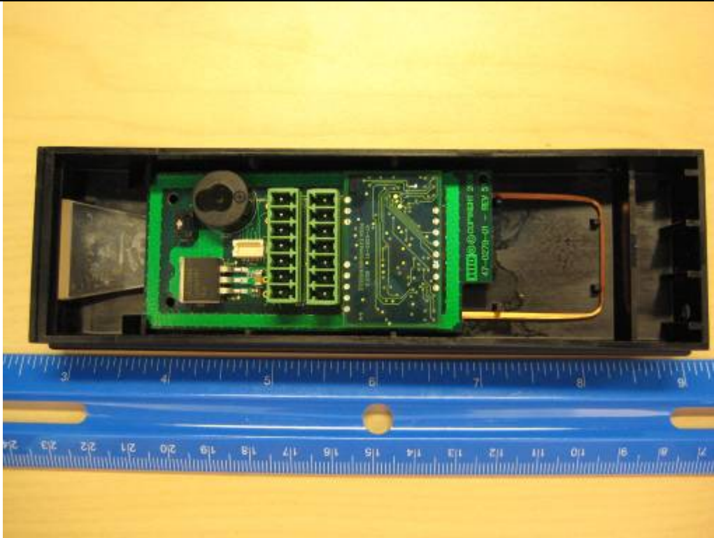
Reader Board in Plastic Housing with Digital I/O Board – Not Potted
