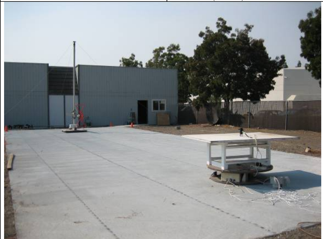
Radiated Emission Test Setup – Rear View (>30MHz)
