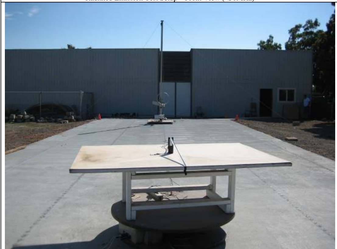
Radiated Emission Test Setup – Rear View (<30MHz)
