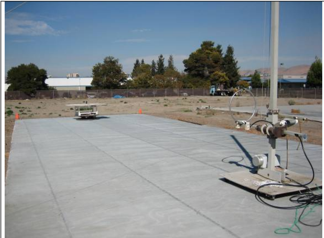
Radiated Emission Test Setup – Front View (<30MHz)
