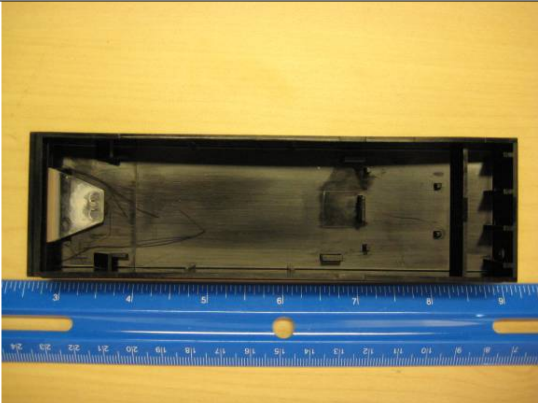
Plastic Housing after Reader Board Removed
