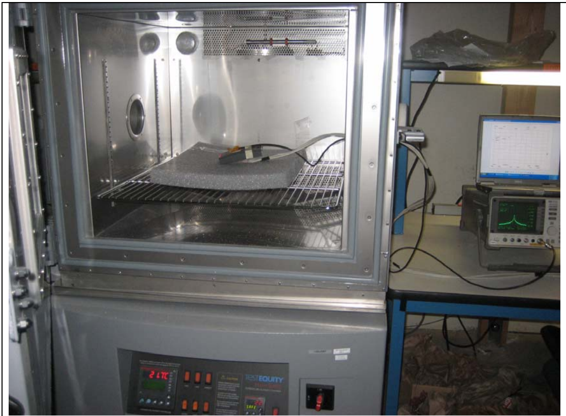
Frequency Stability and Occupied Bandwidth Test Setup – Front View (RP40)
