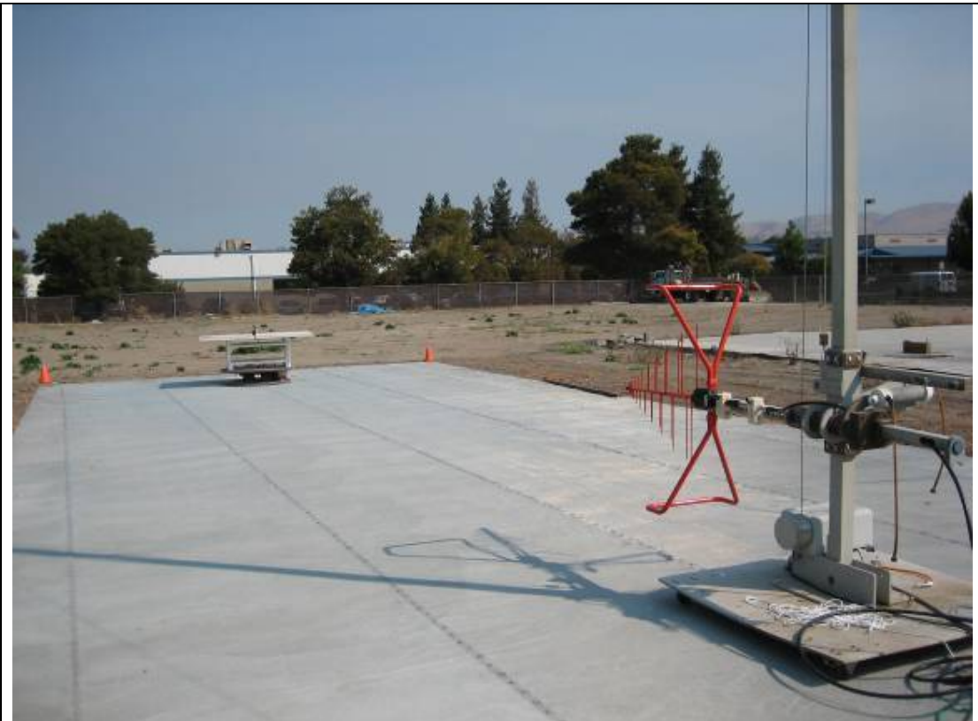
Radiated Emission Test Setup – Front View (>30MHz)
