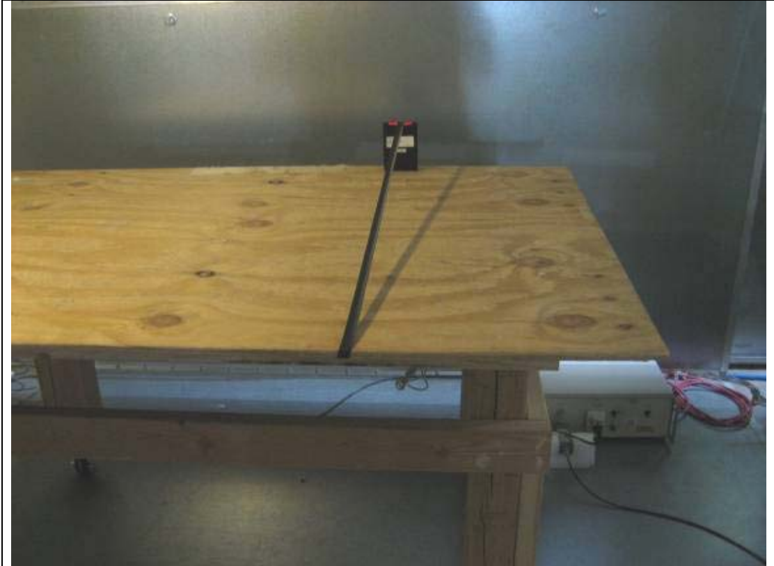
AC Line Conducted Emission Test Setup – Front View 1 (RP40)
