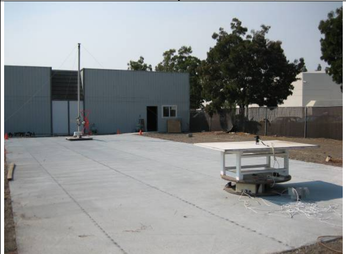
Radiated Emission Test Setup – Rear View (>30MHz)
