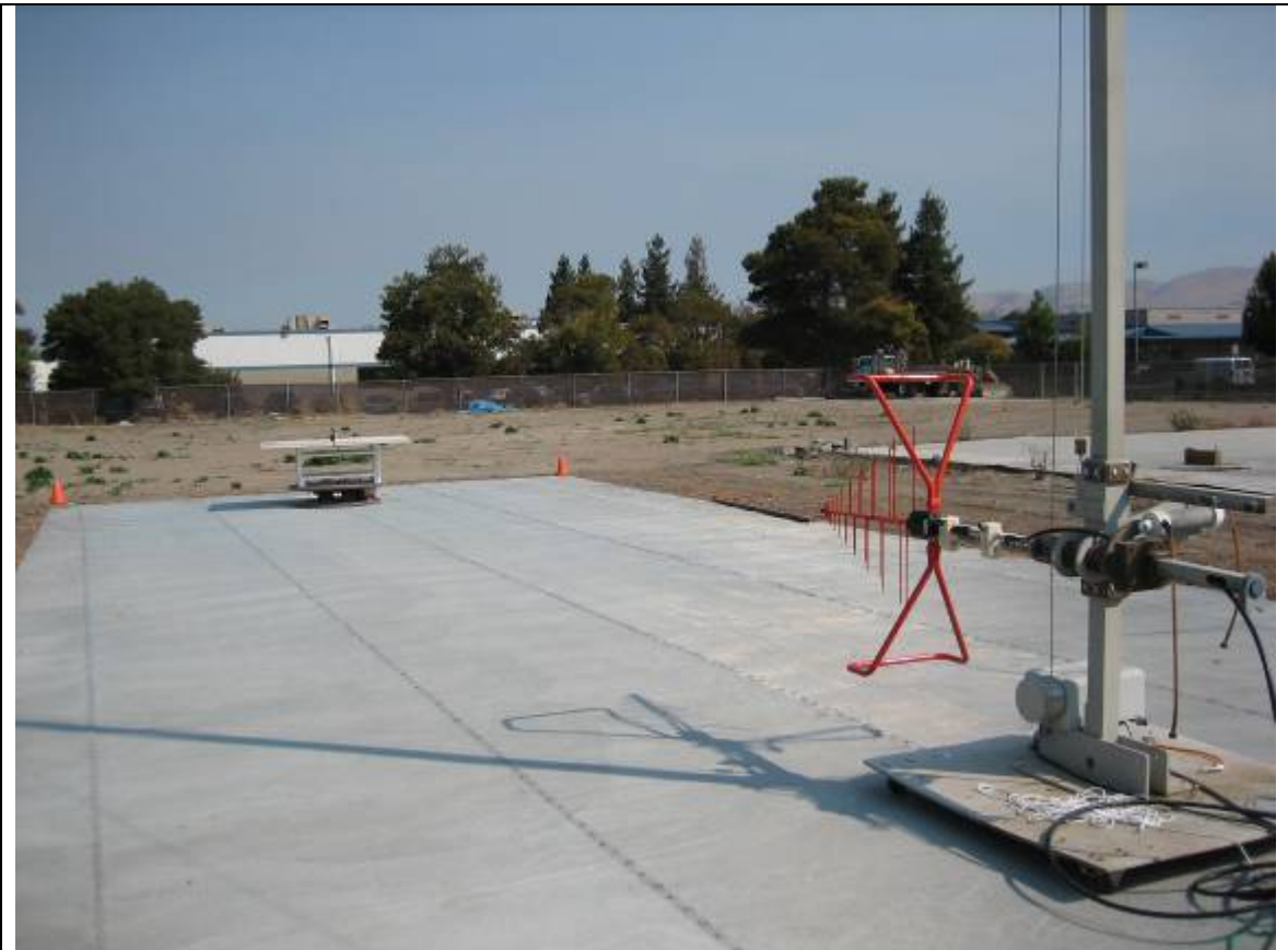
Radiated Emission Test Setup – Front View (>30MHz)
