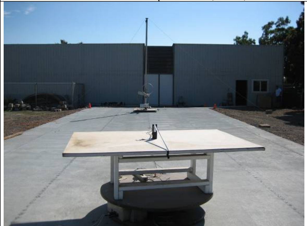
Radiated Emission Test Setup – Rear View (<30MHz)
