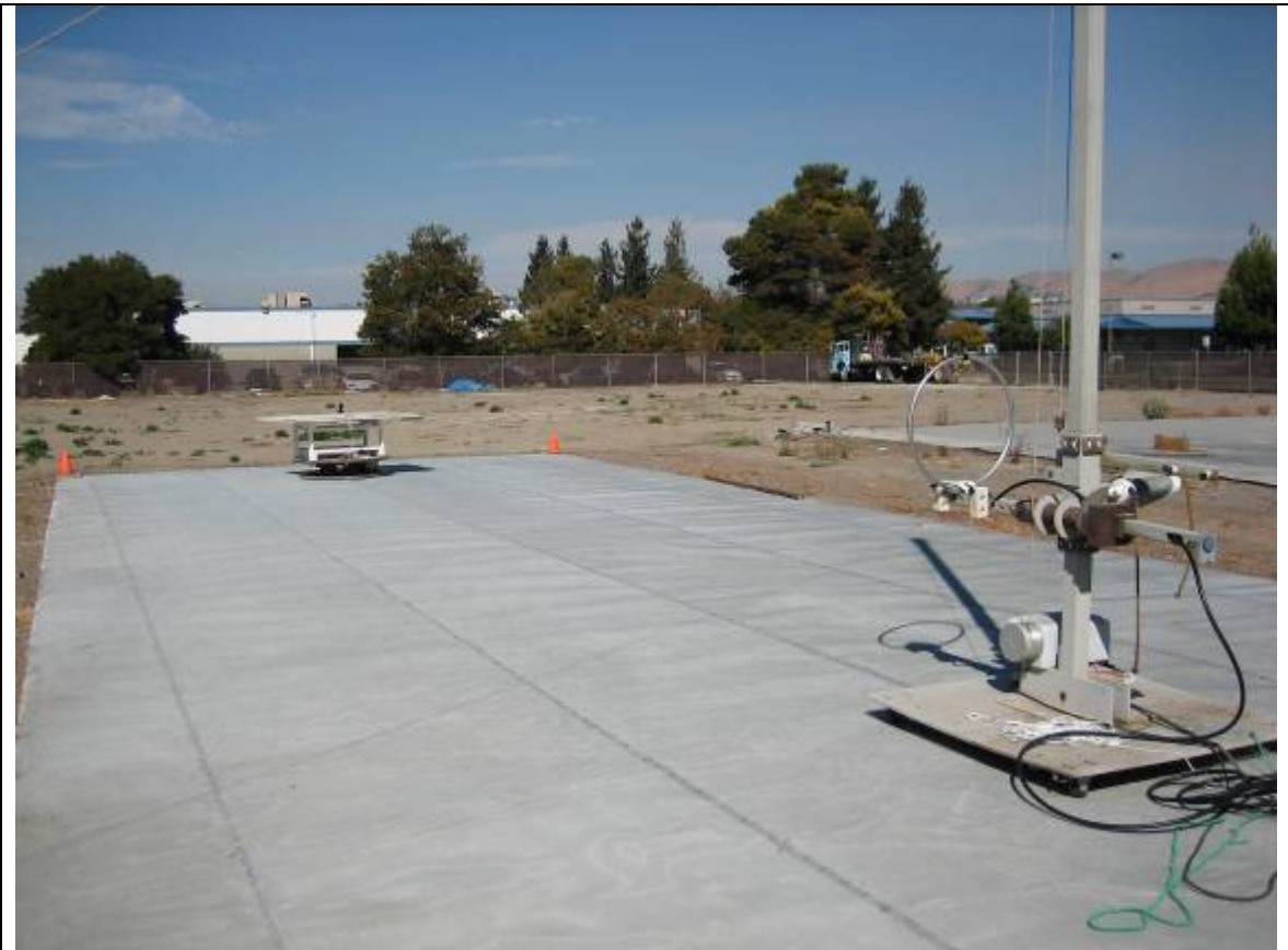
Radiated Emission Test Setup – Front View (<30MHz)
