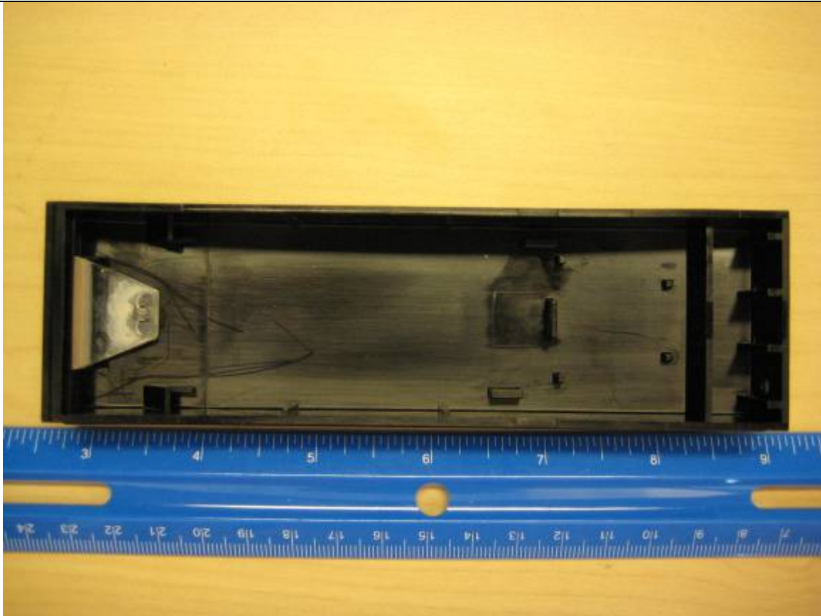
Plastic Housing after Reader Board Removed
