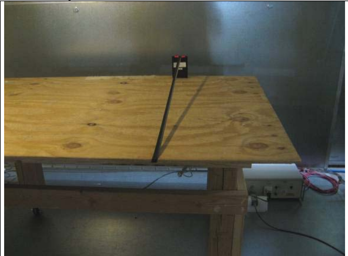
AC Line Conducted Emission Test Setup – Front View
