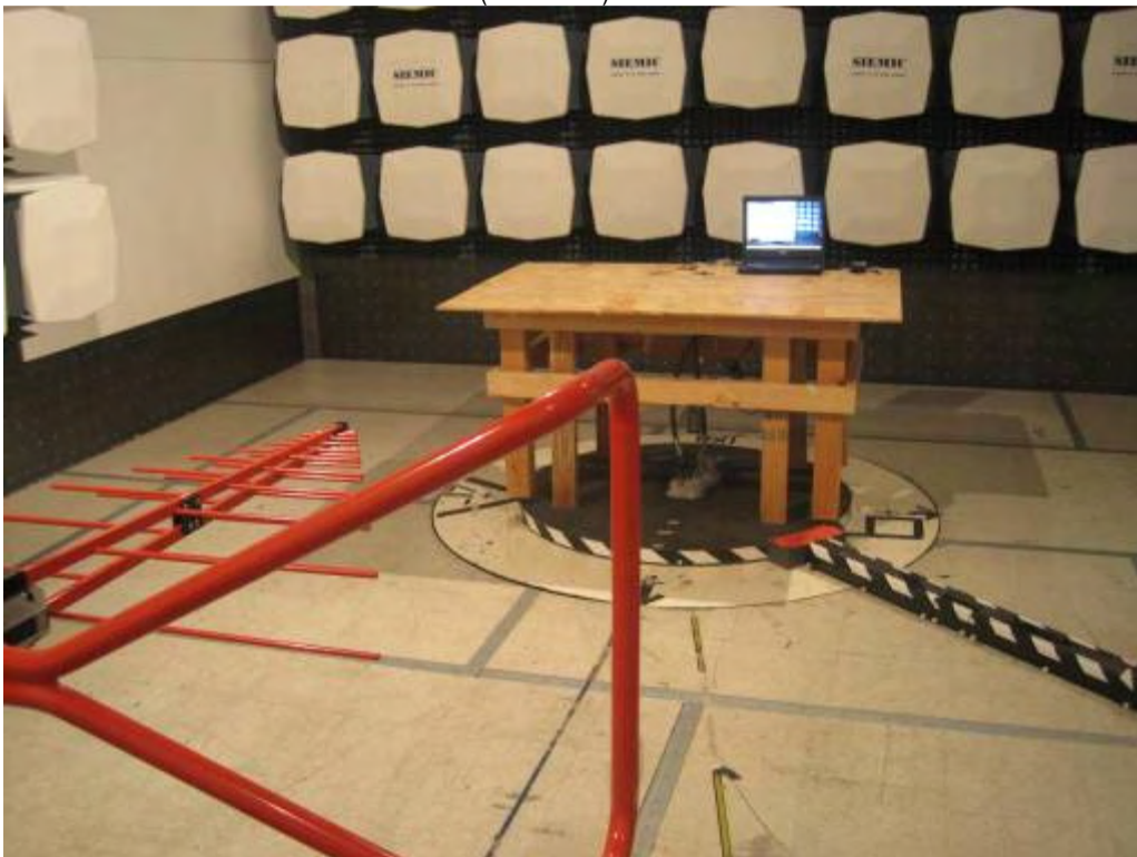
Radiated Emission Test > 30MHz ( Front view) --- identiCLASS 3500 + 2xAntenna ID1
