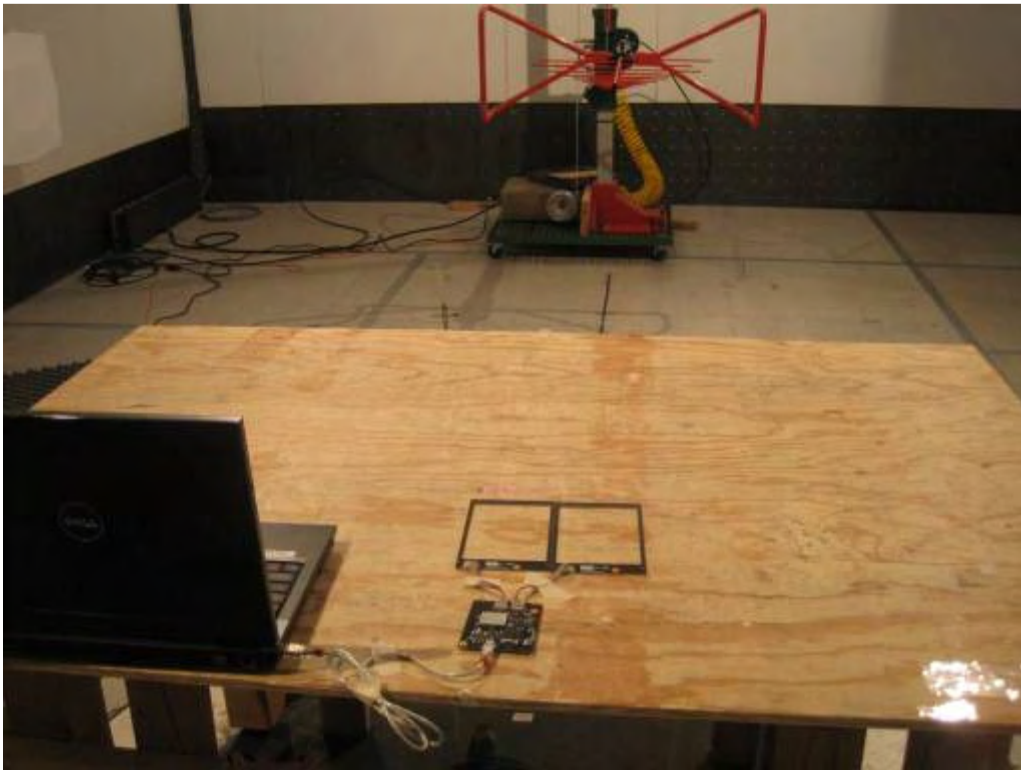
Radiated Emission Test >30MHz ( Rear view) --- identiCLASS 3500 + 2 x Antenna ID3 + SAM ID0
