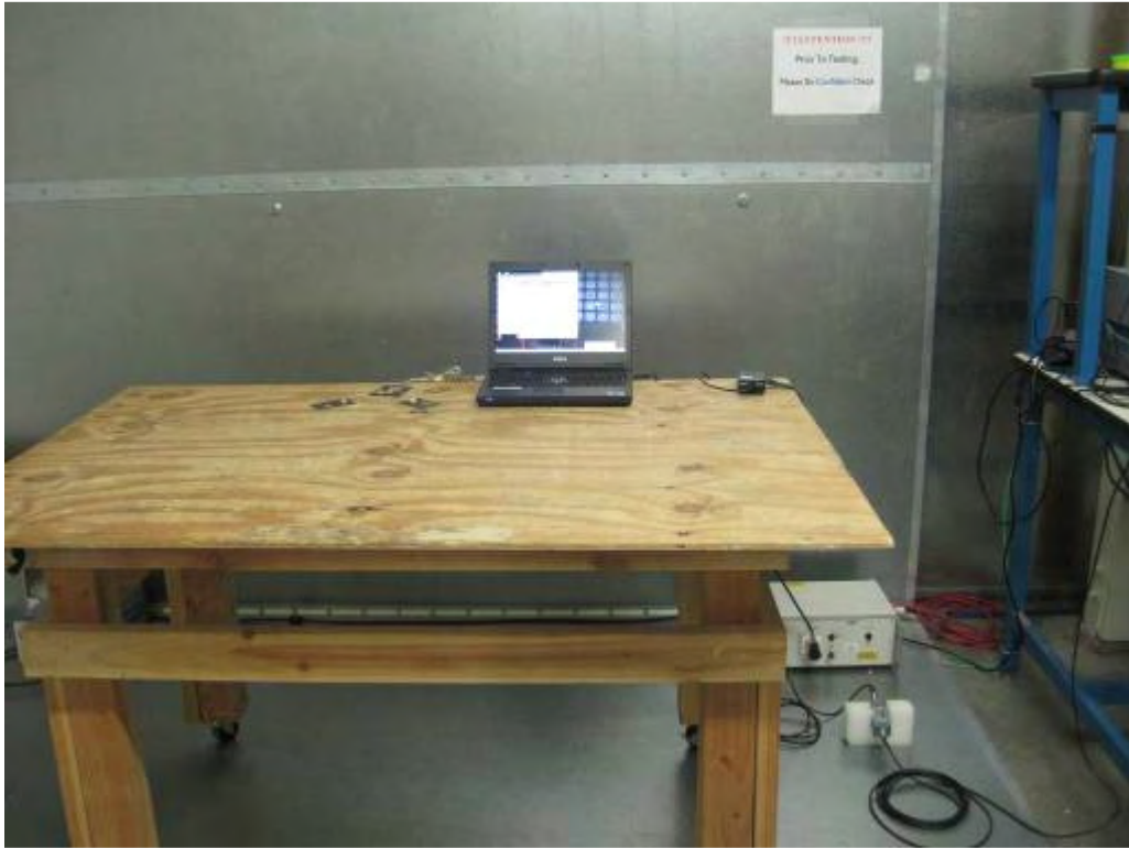
AC Line Conducted Emission Test Setup --- identiCLASS 3500 + 2xAntenna ID1
