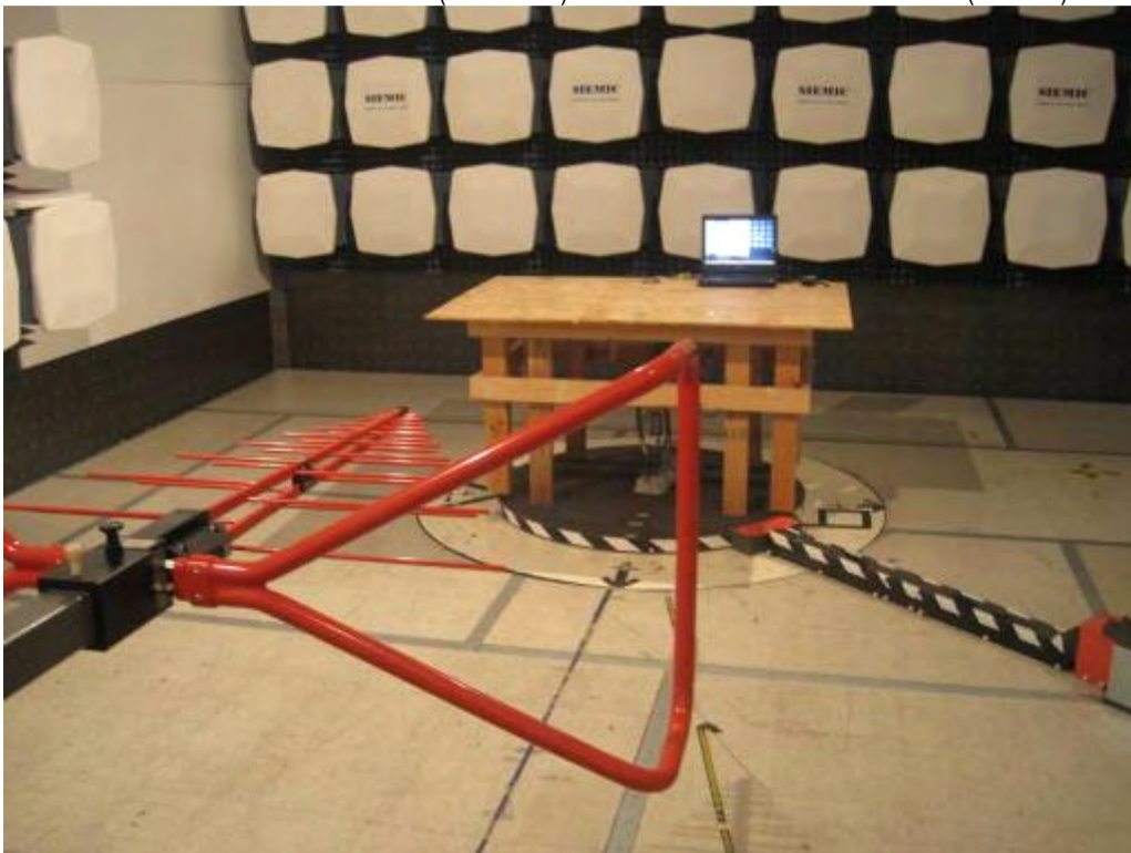
Radiated Emission Test > 30MHz ( Front view ) --- identiCLASS 3500 + Antenna ID0 ( internal )
