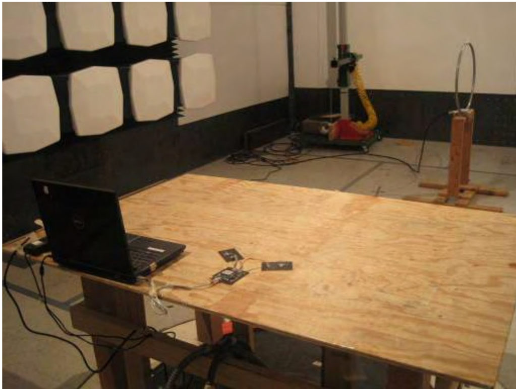
Radiated Emission Test <30MHz ( Rear view) --- identiCLASS 3500 + 2xAntenna ID1
