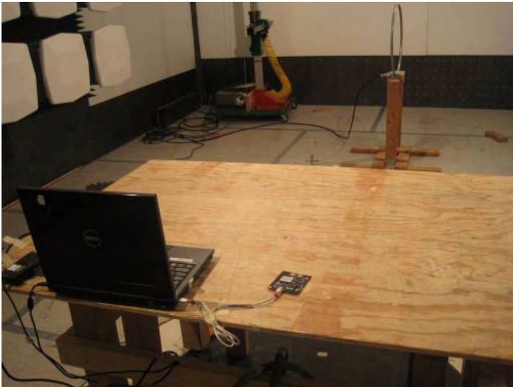
Radiated Emission Test <30MHz ( Rear view) --- identiCLASS 3500 +Antenna ID0 ( internal)
