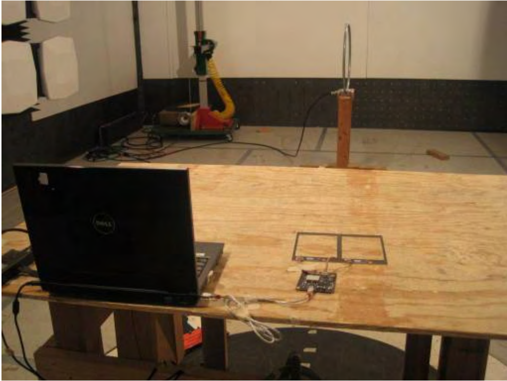
Radiated Emission Test <30MHz ( Rear view) --- identiCLASS 3500 + 2 x Antenna ID3 + SAM ID0
