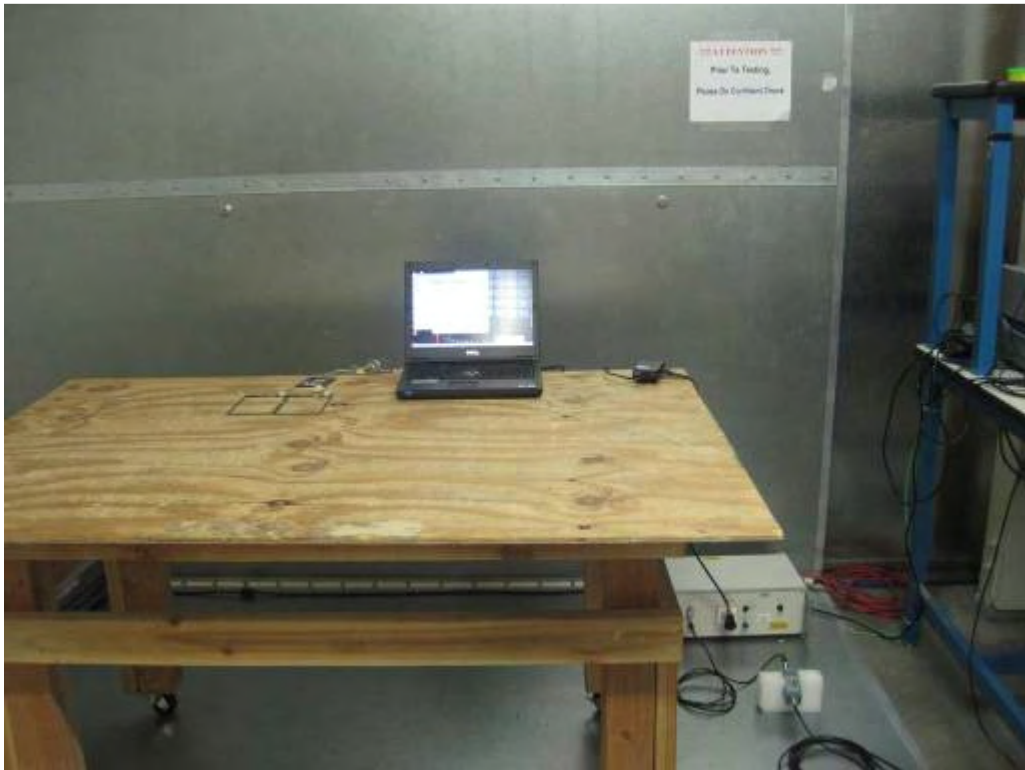
AC Line Conducted Emission Test Setup --- identiCLASS 3500 + 2 x Antenna ID3 + SAM ID0
