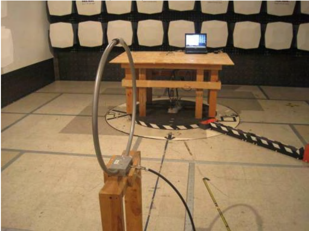
Radiated Emission Test <30MHz ( Rear view) --- identiCLASS 3500 + 2 x Antenna ID3 + SAM ID0
