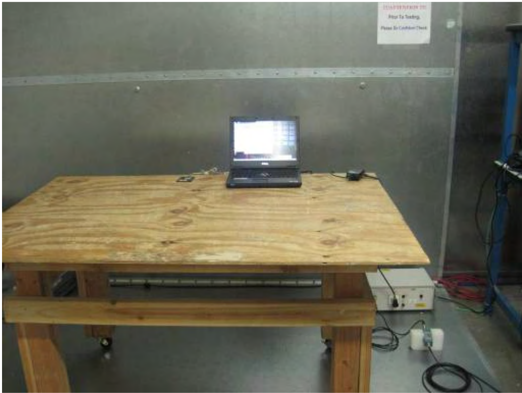
AC Line Conducted Emission Test Setup --- identiCLASS 3500 + Antenna ID0 ( internal)
