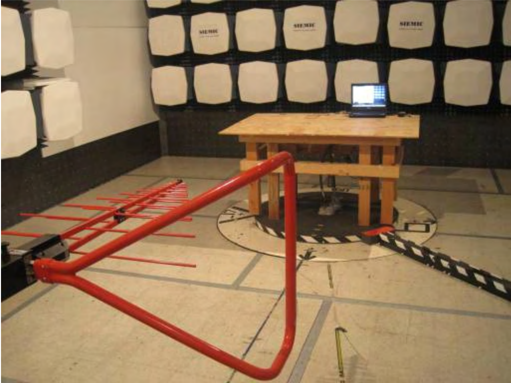
Radiated Emission Test >30MHz (Rear View) --- identiCLASS 3300 + Antenna ID3 + SAM ID0
