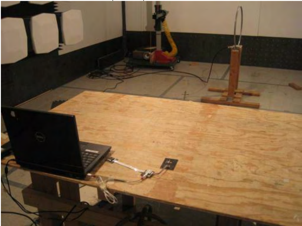
Radiated Emission Test <30MHz (Rear View) --- identiCLASS 3300 + Antenna ID1 + SAM ID0
