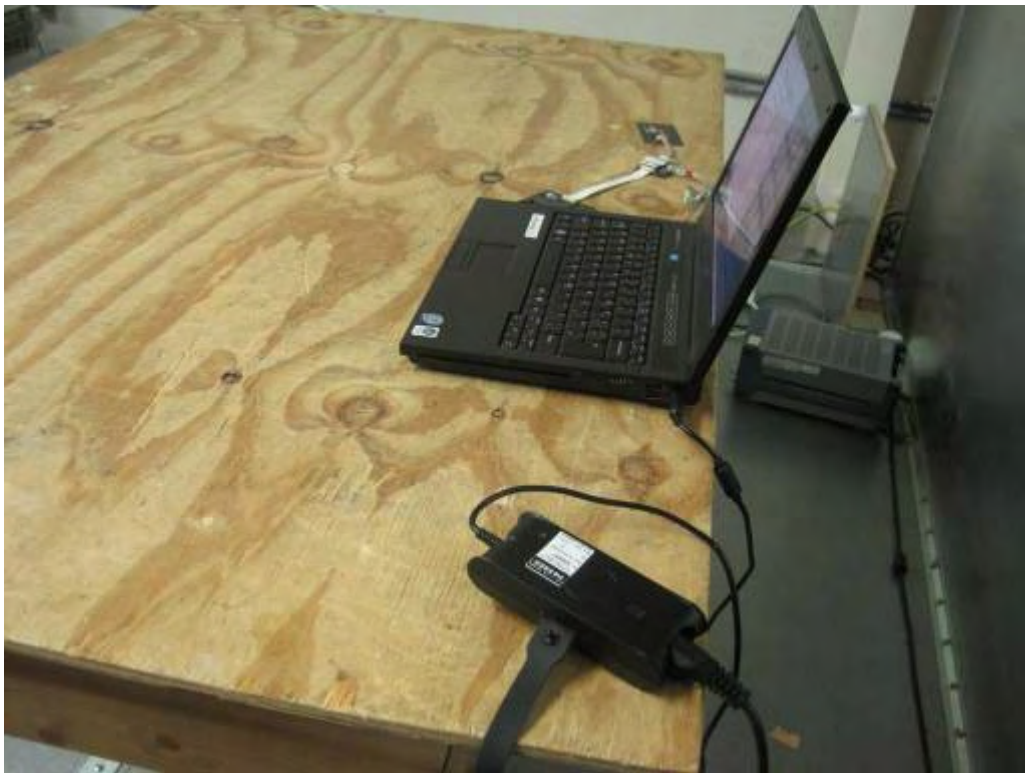
AC Line Conducted Emission Rear View -- identiCLASS 3300 + Antenna ID1 + SAM ID0
