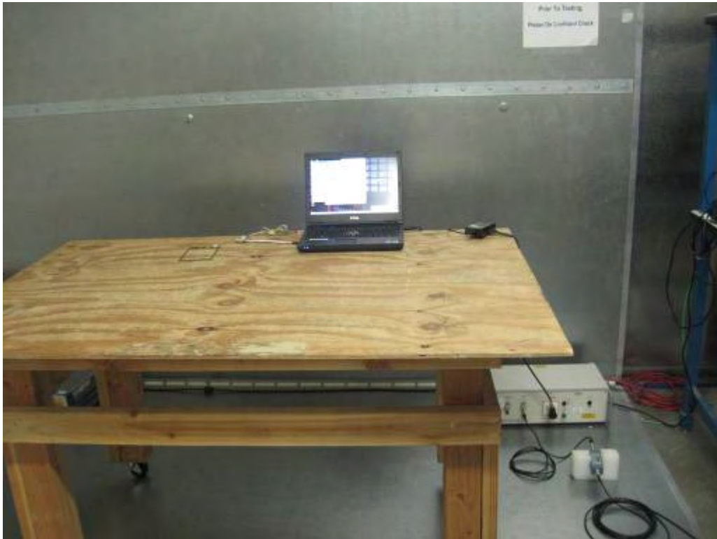
AC Line Conducted Emission Front View -- identiCLASS 3300 + Antenna ID3 + SAM ID0
