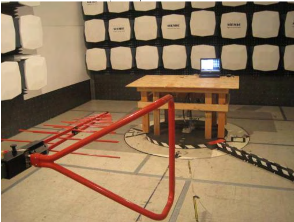
Radiated Emission Test >30MHz (front View) --- identiCLASS 3300 + Antenna ID1 + SAM ID0
