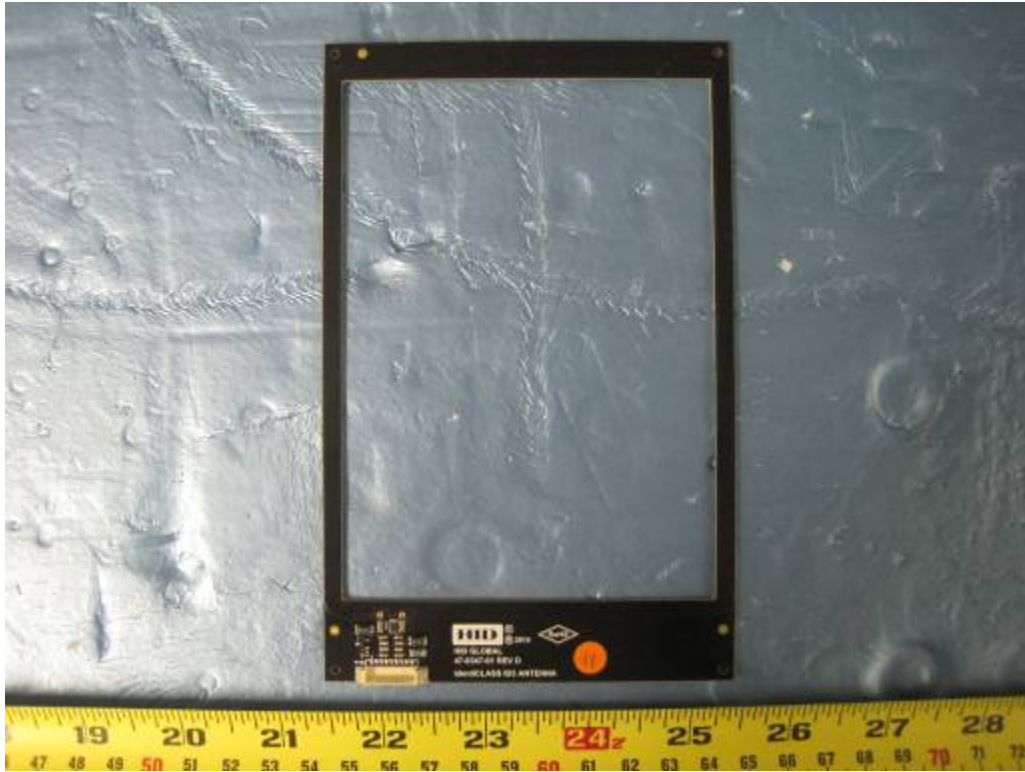
Antenna ID3 Top View
