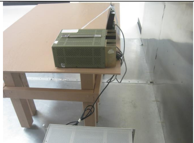
AC Line Conducted Emissions – Rear View
