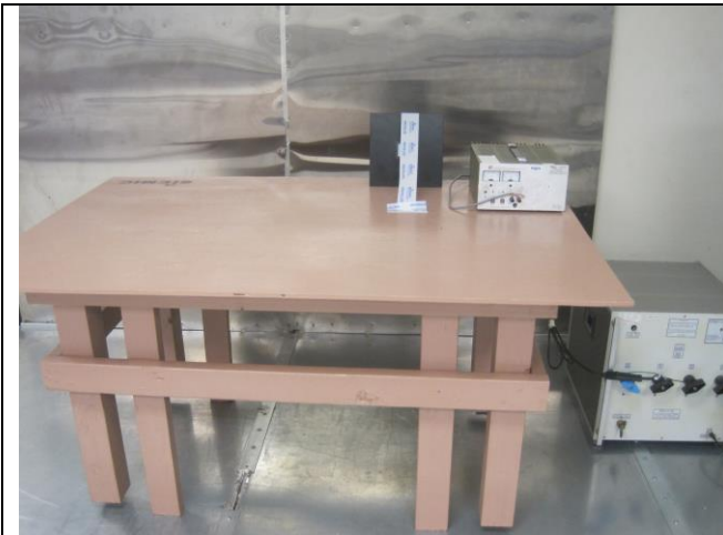
AC Line Conducted Emissions – Front View
