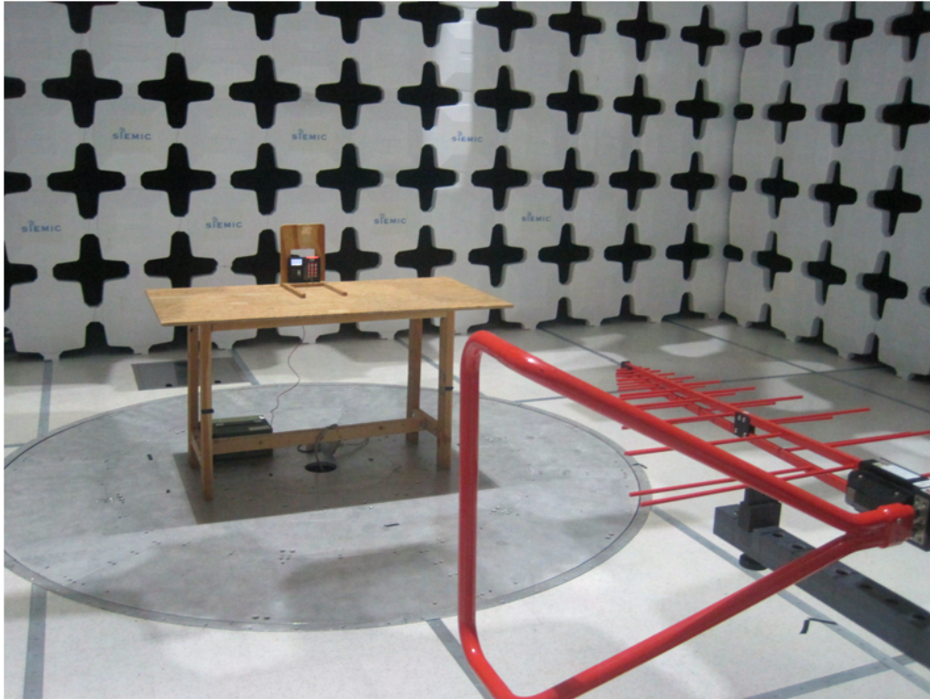
Radiated Emission >30MHz Test Setup – Front View
