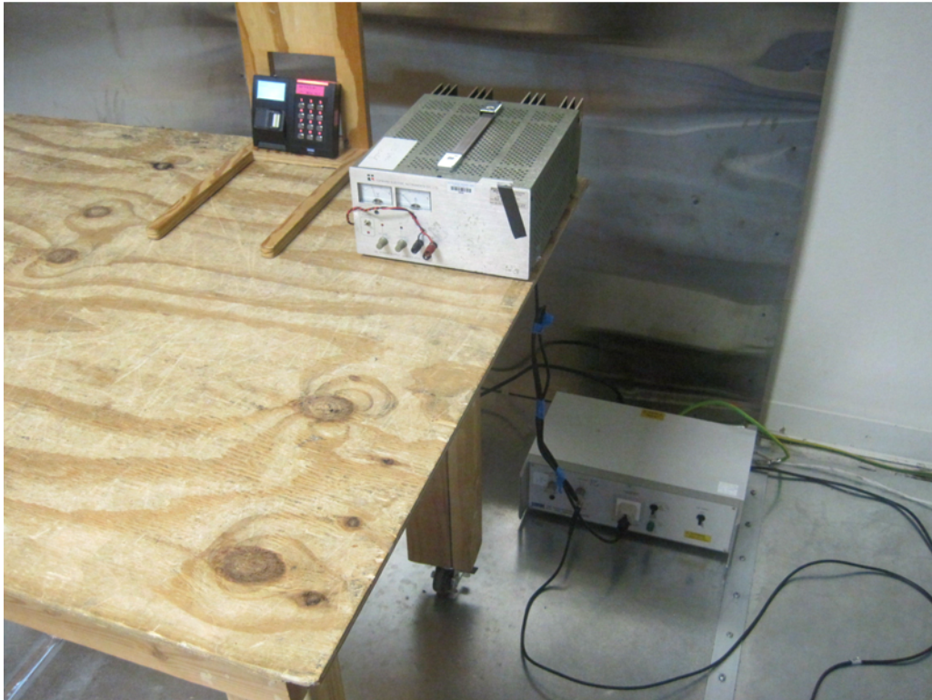
Conducted Emission Test Setup – Front View
