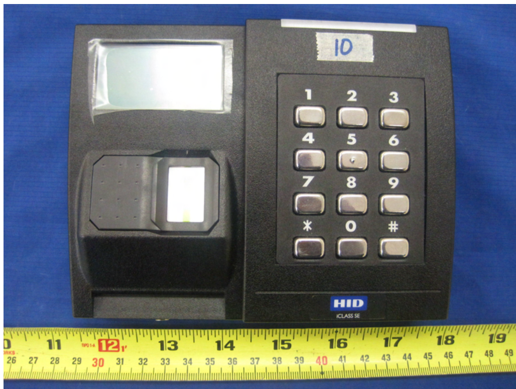
EUT with RFID reader Top View
