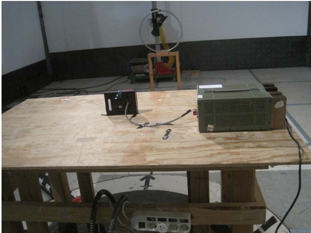
Radiated Emission<30MHz Test Setup – Rear View
