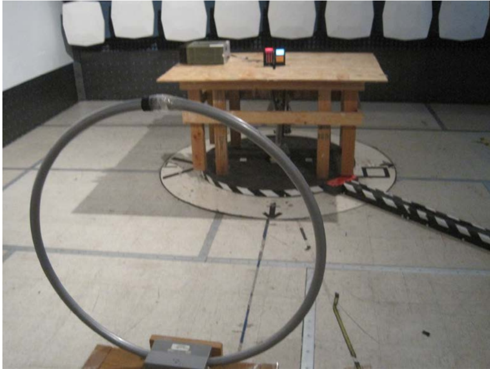
Radiated Emission<30MHz Test Setup – Front View
