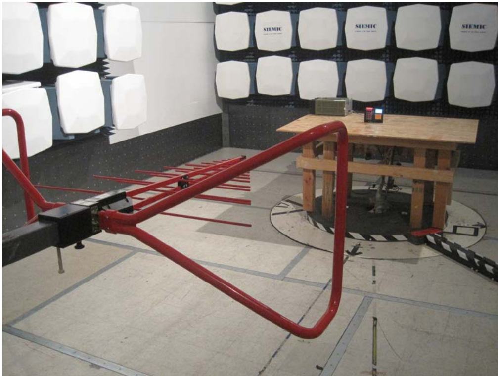
Radiated Emission>30MHz Test Setup – Front View
