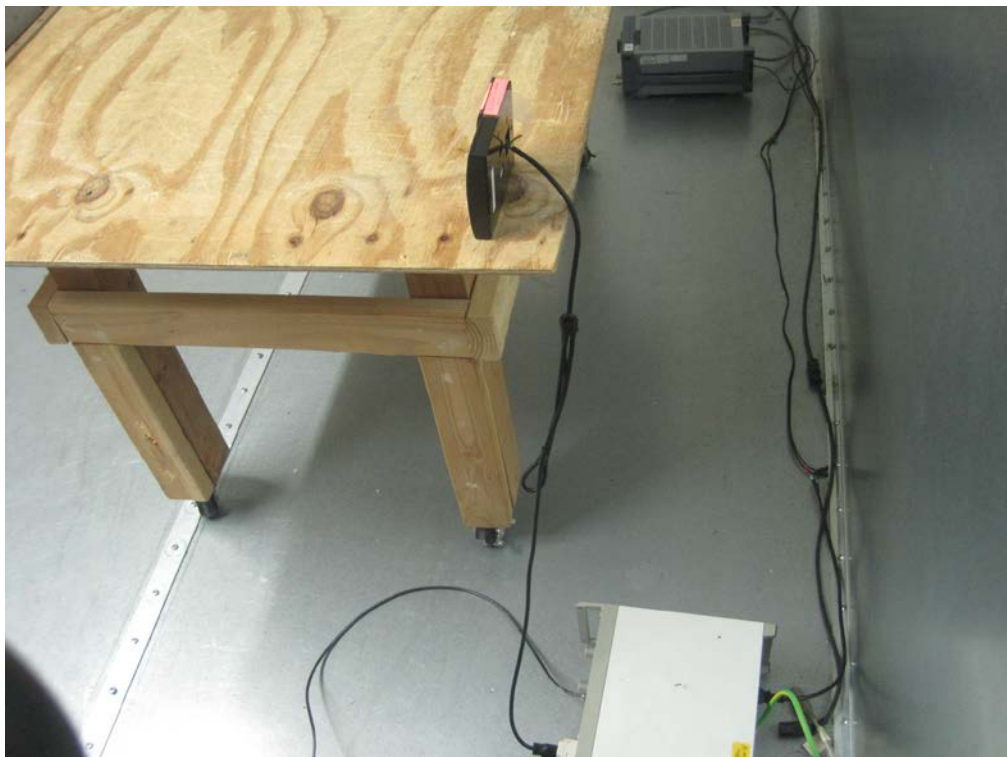
Conducted Emission Test Setup – Rear View
