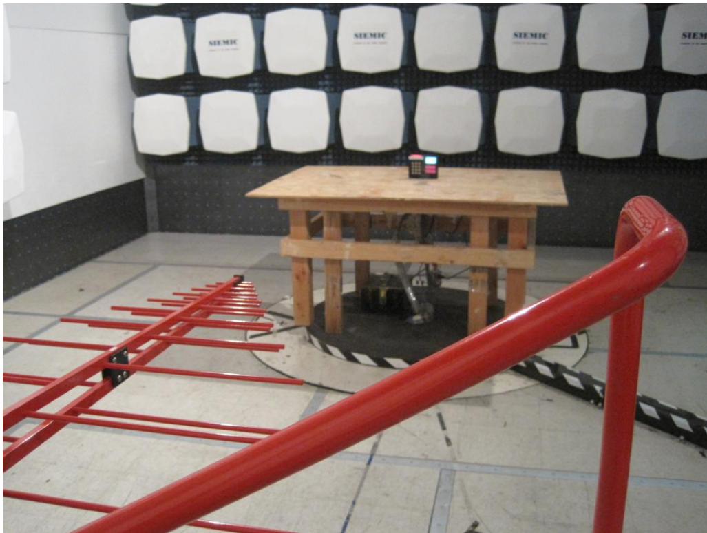
Radiated Emission Test Setup – Front View (Terminal Connectors)
