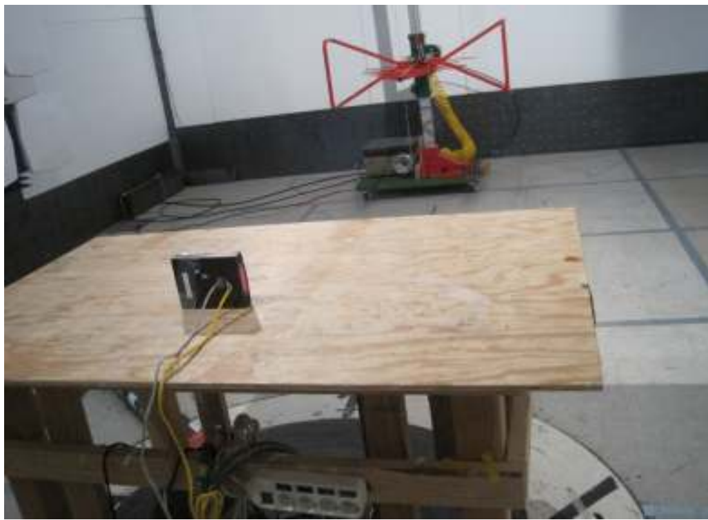
Radiated Emission Test Setup – Rear View (Terminal Connectors)
