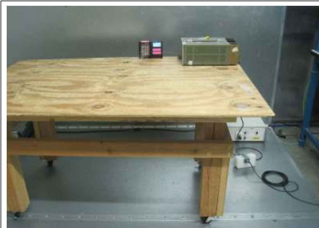
Conducted Emission Test Setup – Front View ( Pig-Tail Connectors)
