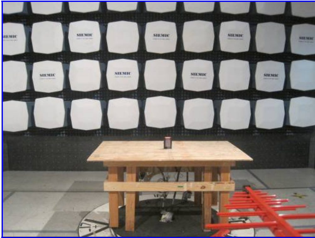
Radiated Emission, Model RK40D (>30MHz) – Front View
