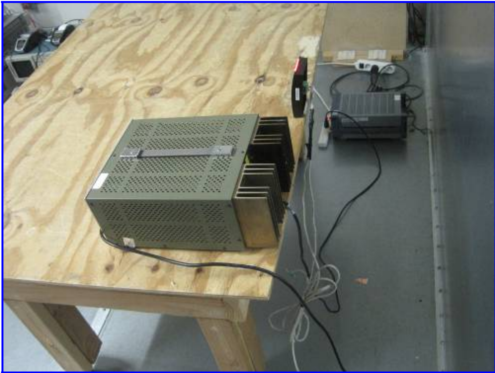
AC Line Conducted Emission Set up 1, Model RK40D - Front View
