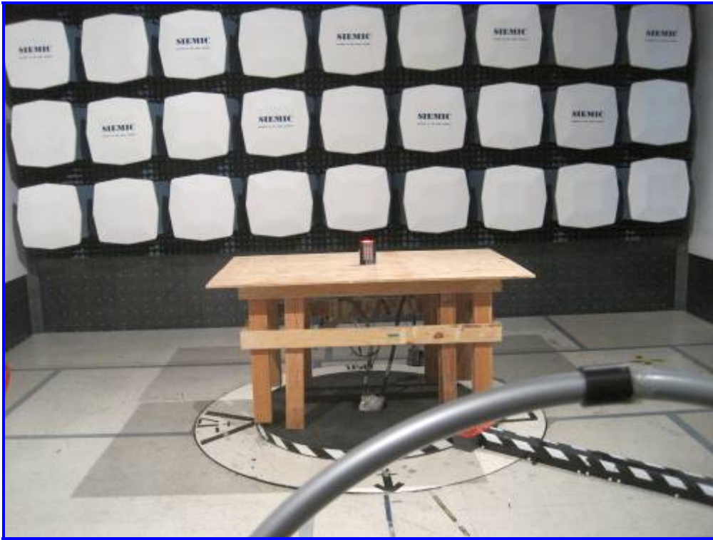
Radiated Emission, Model RK40D (<30MHz) – Front View
