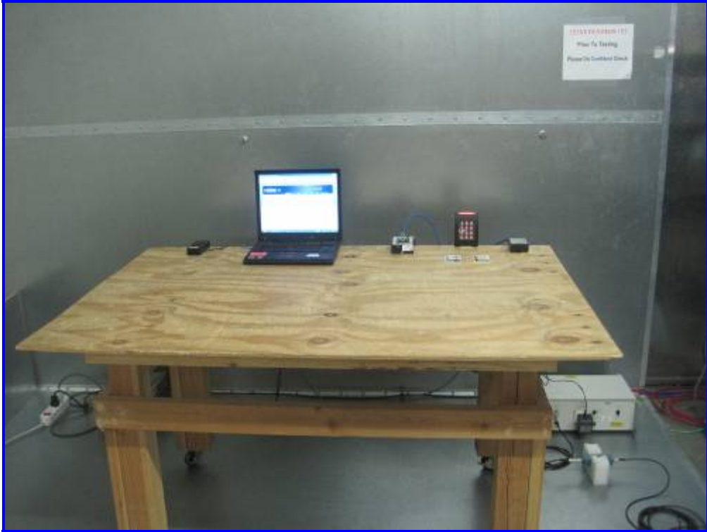
AC Line Conducted Emission Set up 2, Model RK40D - Front View
