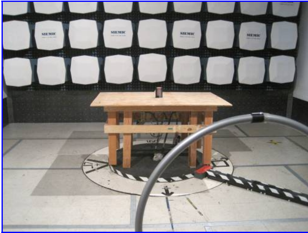
Radiated Emission, Model RK40D (<30MHz) – Front View
