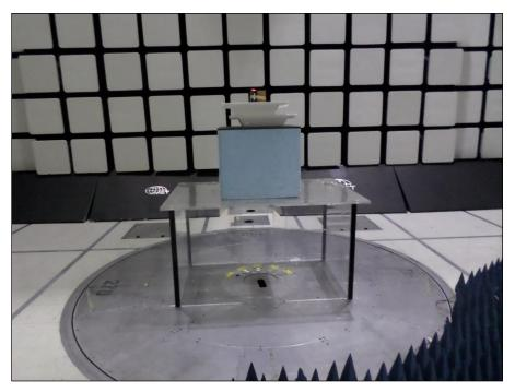
Photograph 9. Radiated Emissions, Setup Above 1 GHz, Front
