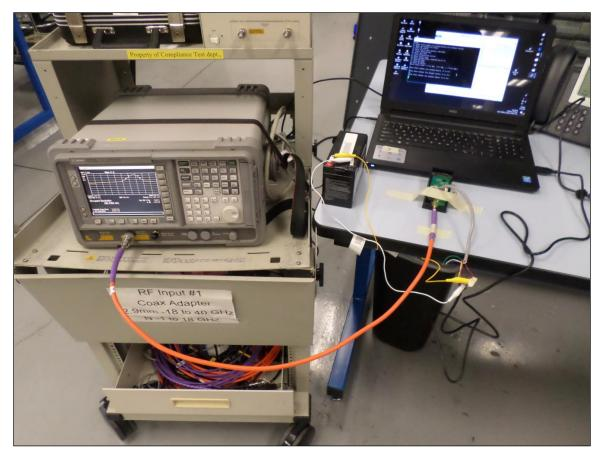
Photograph 3. Occupied Bandwidth, Conducted Testing Setup
