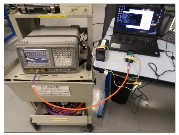
Photograph 15. Power Density, Conducted Testing Setup
