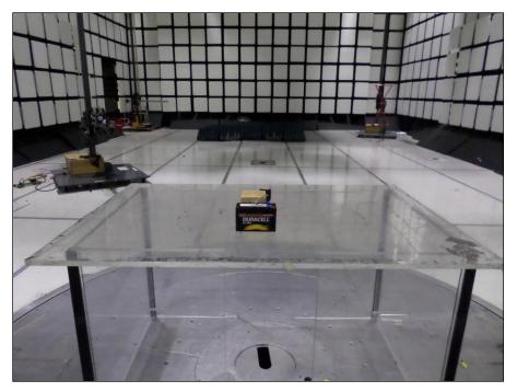
Photograph 7. Radiated Emissions, 30 MHz – 1 GHz, Rear
