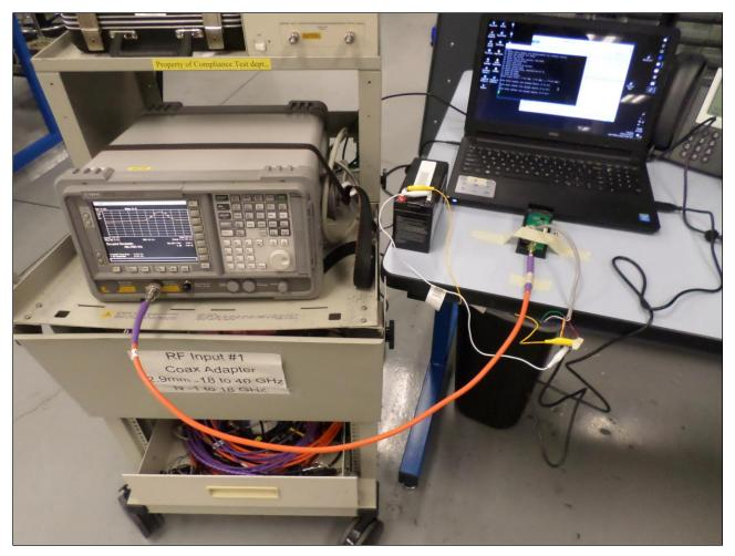
Photograph 14. Conducted Spurious Emissions, Conducted Testing Setup
