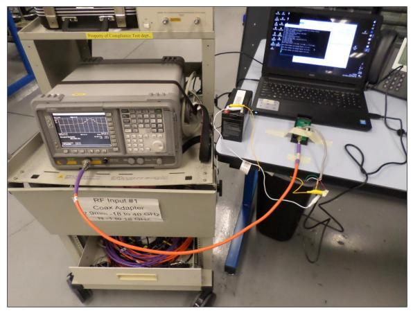
Photograph 4. Peak Power Output, Conducted Testing Setup
