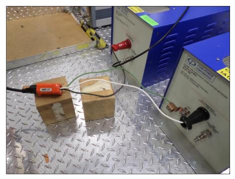
Photograph 2. Conducted Emissions, 15.207(a), LISN Setup
