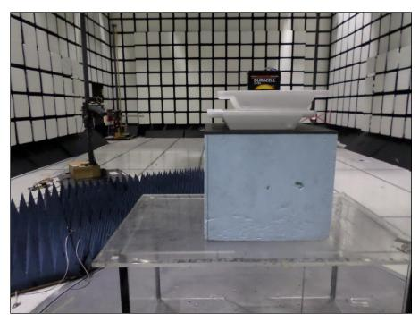
Photograph 10. Radiated Emissions, Setup Above 1 GHz, Rear
