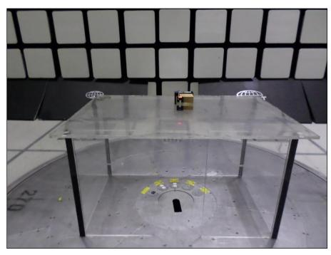
Photograph 6. Radiated Emissions, 30 MHz – 1 GHz, Front
