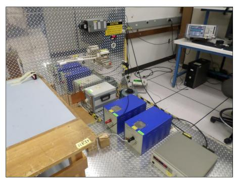
Photograph 1. Conducted Emissions, 15.207(a), Test Setup
