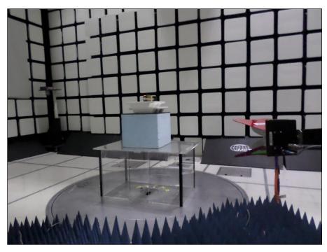
Photograph 8. Radiated Emissions, Setup Above 1 GHz, Antenna
