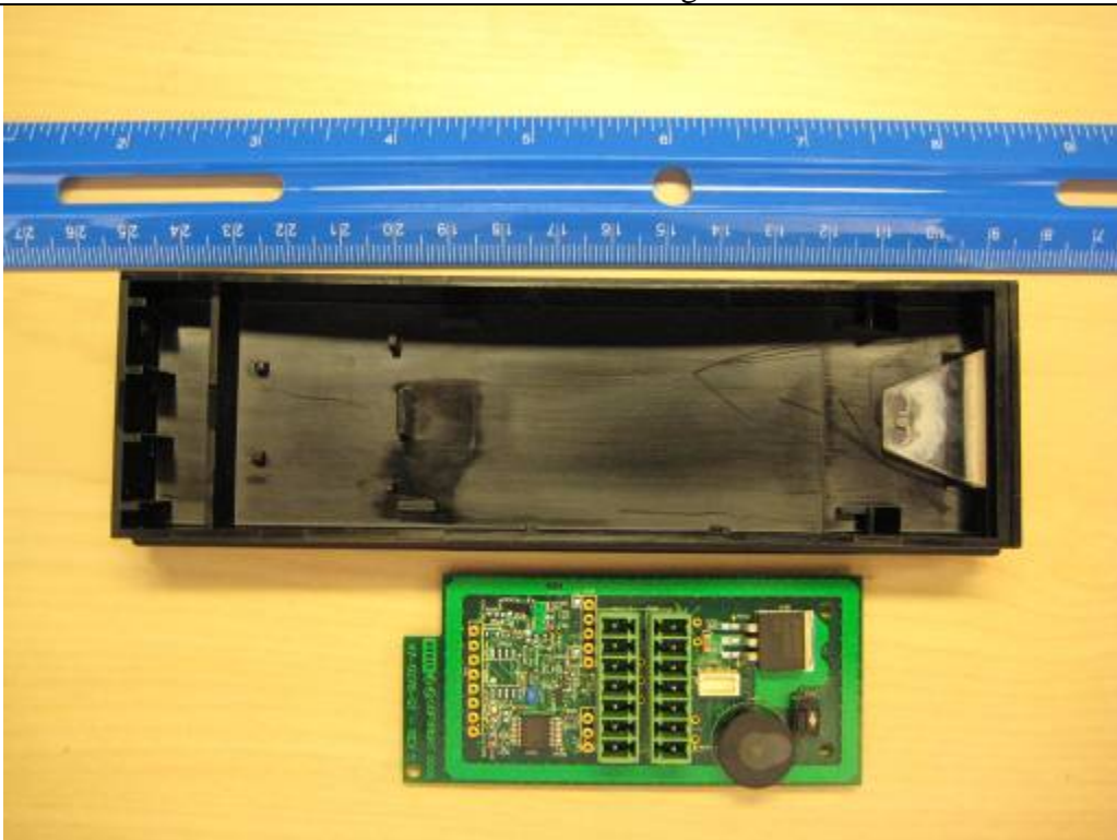
Plastic Housing after Reader Board Removed
