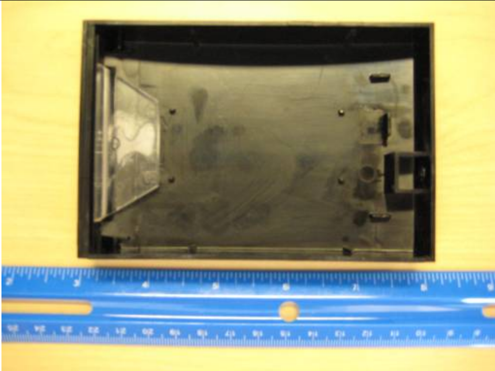
Plastic Housing after Reader Board Removed
