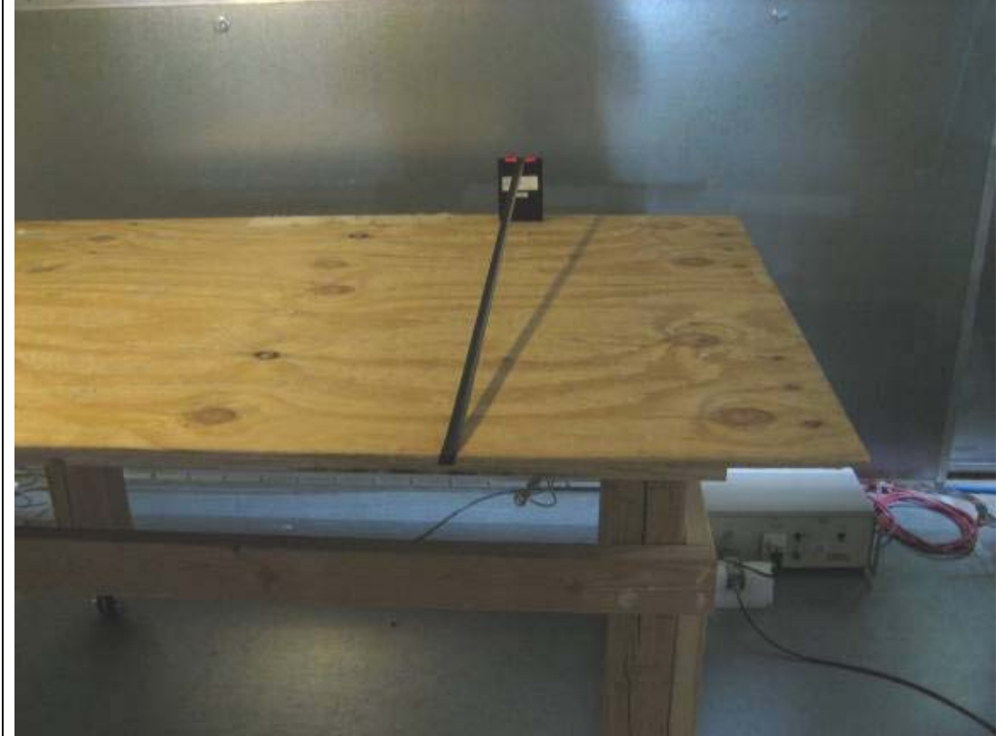
AC Line Conducted Emission Test Setup – Front View 1 (R40)
