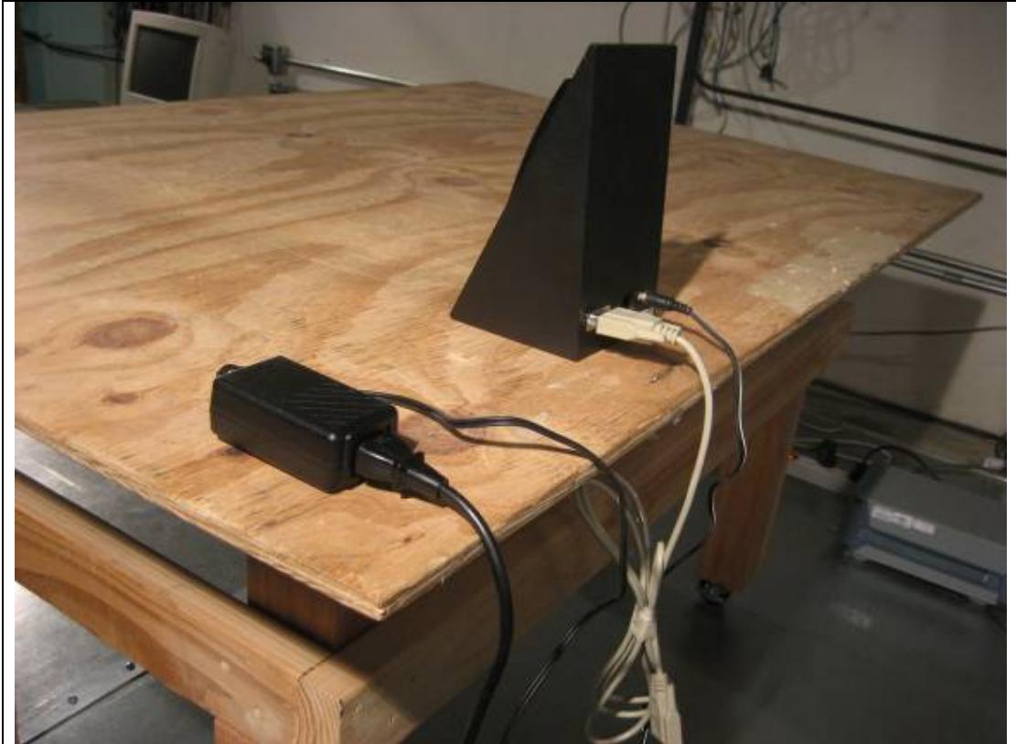
AC Line Conducted Emission Test Setup – Rear View (CP400-R40 on a plastic base)
