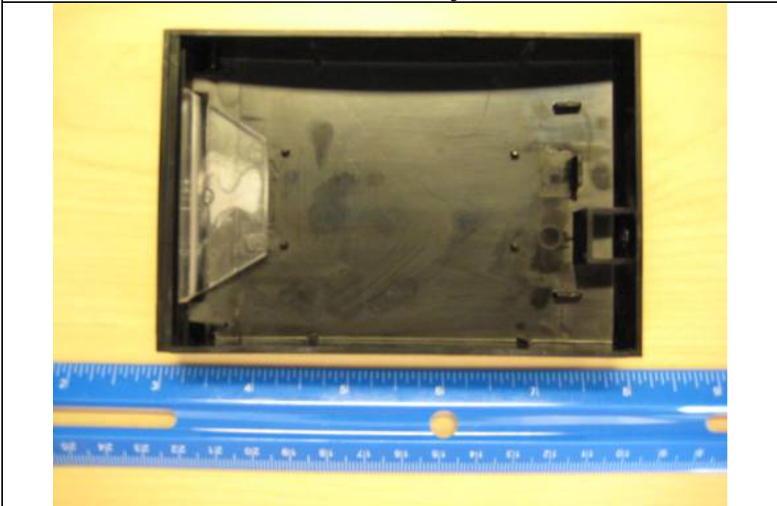
Plastic Housing after Reader Board Removed
