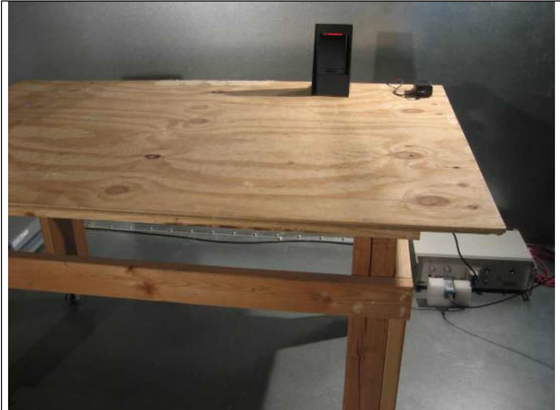
AC Line Conducted Emission Test Setup – Front View (CP400-R40 on a plastic base)
