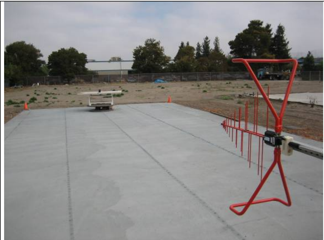
Radiated Emission Test Setup – Front View (>30MHz)
