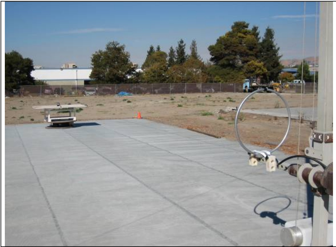
Radiated Emission Test Setup – Front View (<30MHz)
