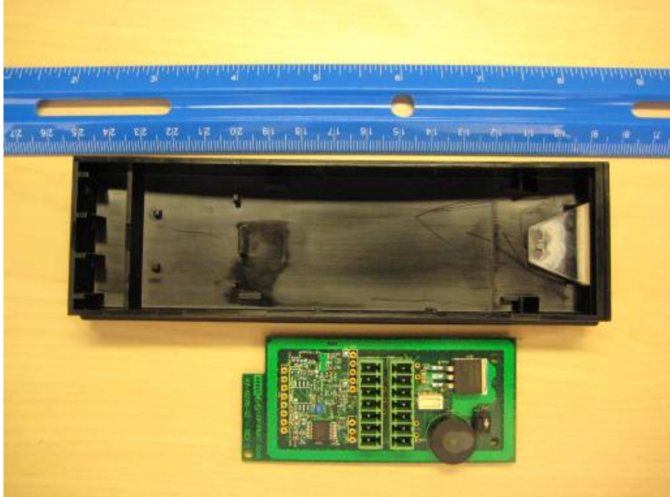
Plastic Housing after Reader Board Removed
