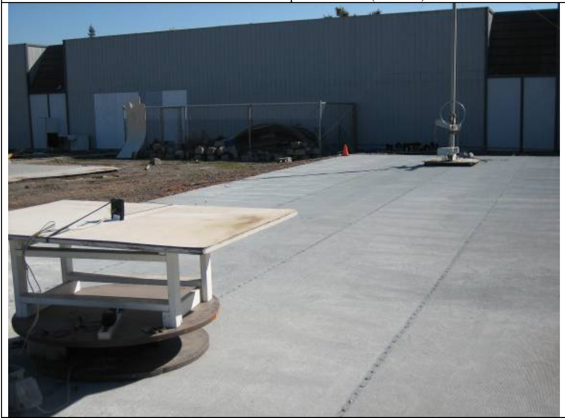
Radiated Emission Test Setup – Rear View (<30MHz)
