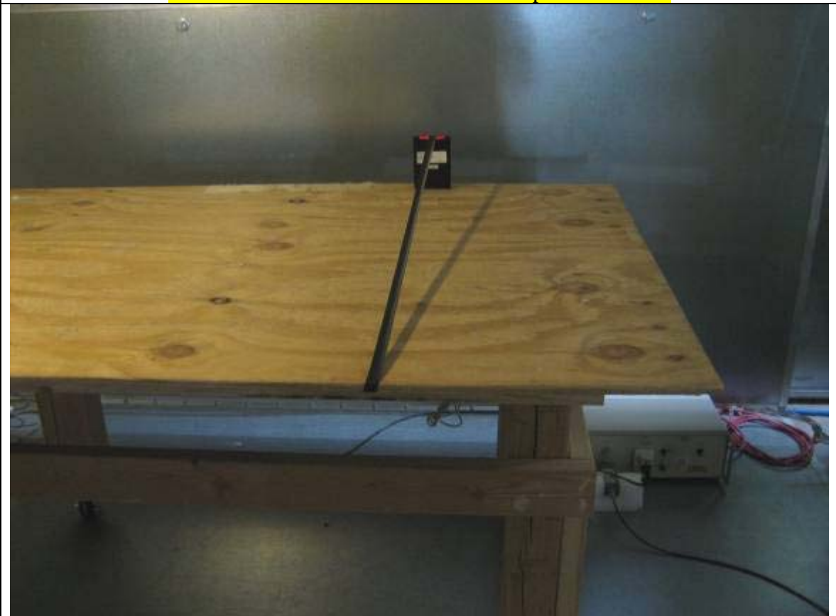
DC Line Conducted Emission Test Setup – Front View
