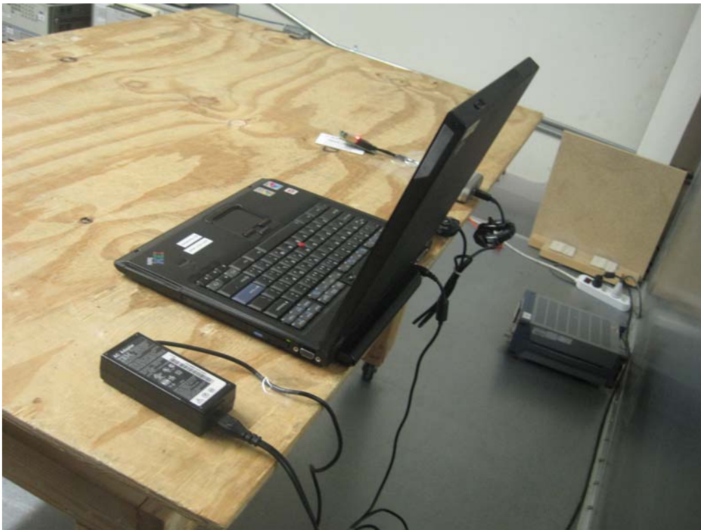
AC Line Conducted Emission Rear View
