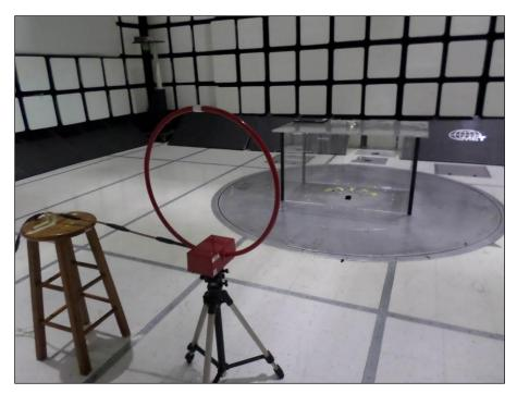
Photograph 1. Radiated Emissions, 0.009 MHz – 1.250 MHz, Antenna View
