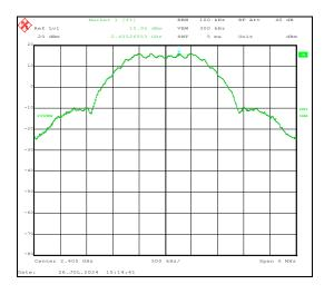
The peak level of 16 dBm is the maximum peak output of the Lutron Model RRL-MWCL LED Lighting Controller. The conducted spurious emissions from the antenna port must be 20 dB down from this peak. The resultant limit is therefore -4.0 dBm and is displayed on the plots below.
