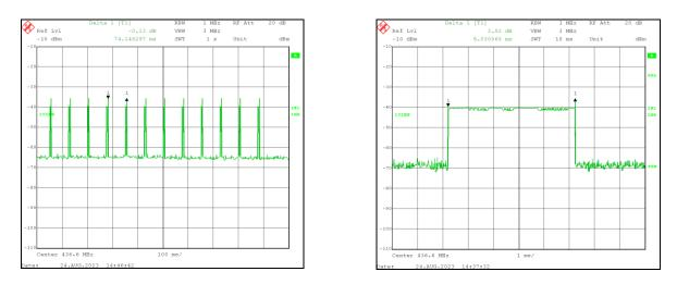
The measured on-times depicted on the spectrum analyzer screens above are used to calculate the Duty Cycle Correction Factor. This factor is used to reduce the emission level of spurious emissions measured and displayed in Section 4.3.
