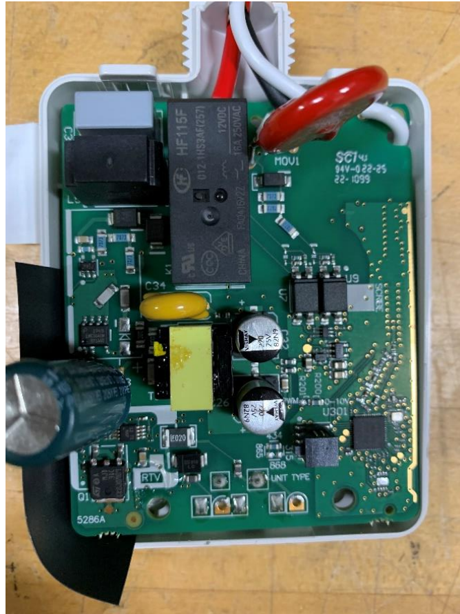
PWB Back with Cap and MOV Lifted
