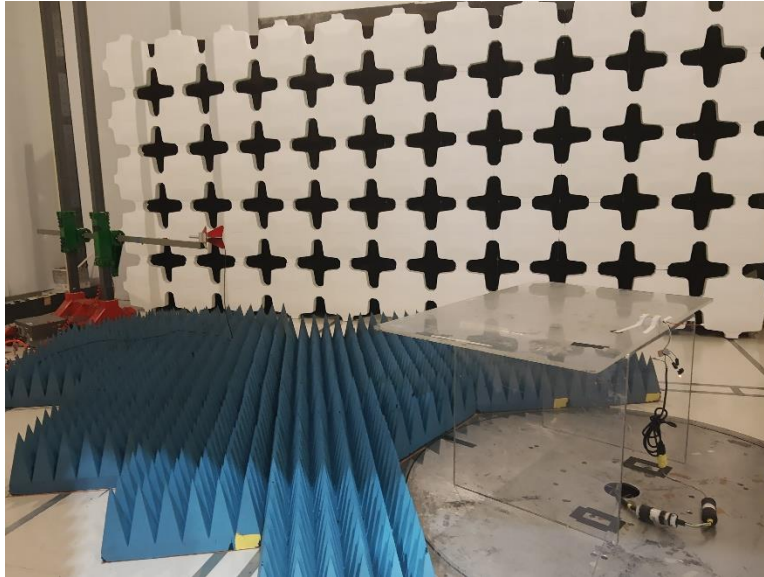
Photograph 3. RE Above 1GHz Test Setup
