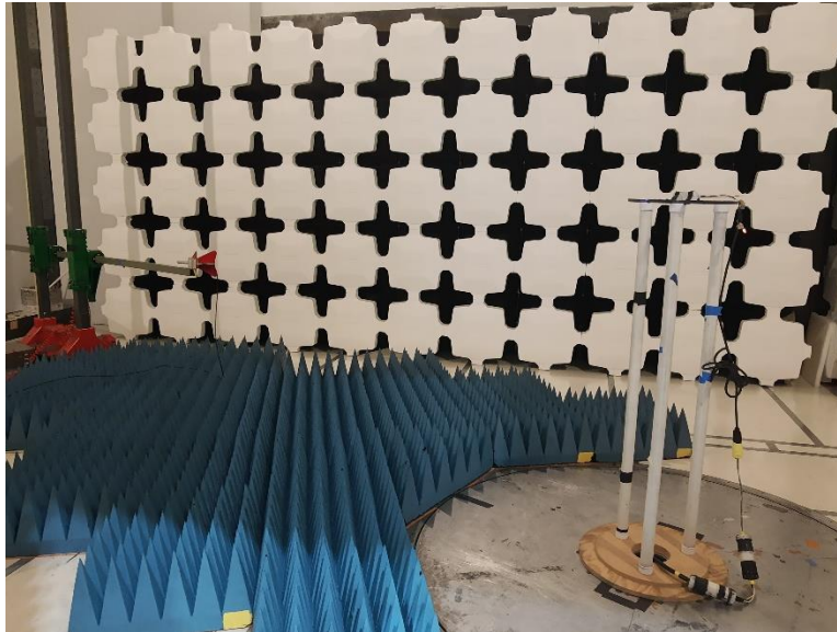
Photograph 3. Radiated Emissions Test Setup, 1-5 GHz
